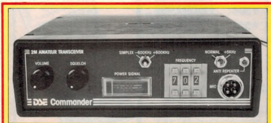
Above: Complete two-metre transceiver built from a kit and (below) an interior view of the same set (EA June/July 84). Building a set like this not only saves money, but provides the builder with invaluable experience.
