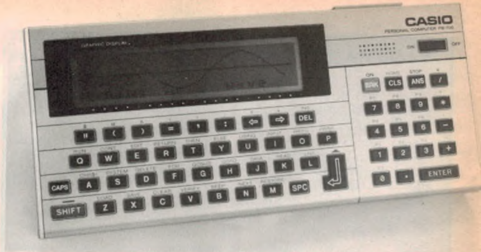
The Casio PB-700 can be used to generate graphic displays as this sine plot shows.
