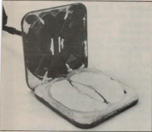
Inside the search head. The transmit and receive coils overlap by about 25mm.
