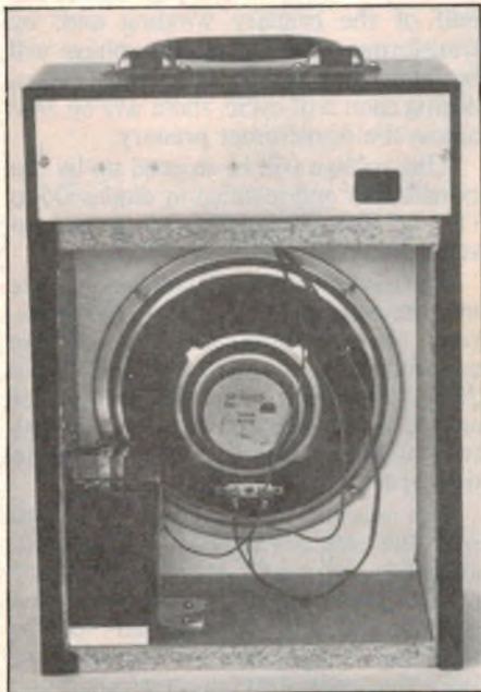
Rear view of the Busker. The battery holder is made from scrap aluminium.
