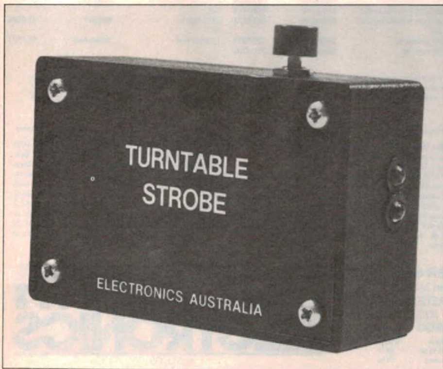
The Turntable Strobe uses a crystal-controlled 100Hz oscillator to drive two high-brightness LEDs. Prototype was housed in a plastic zippy case.
