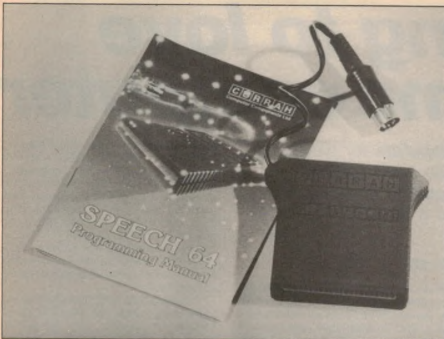
The Speech 64 plugs into the cartridge expansion slot on the back of the Commodore 64.
