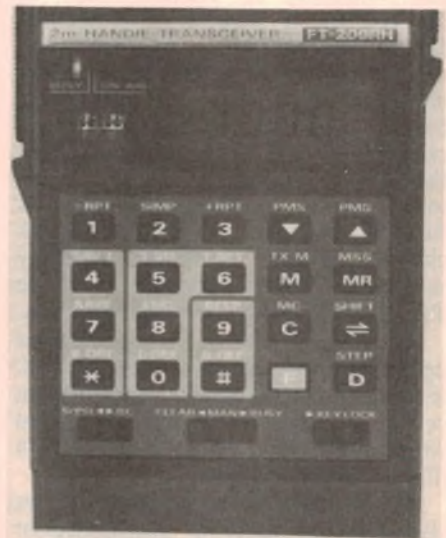
This 20-button keypad controls most the operating functions, provides a seemingly endless list of facilities.
