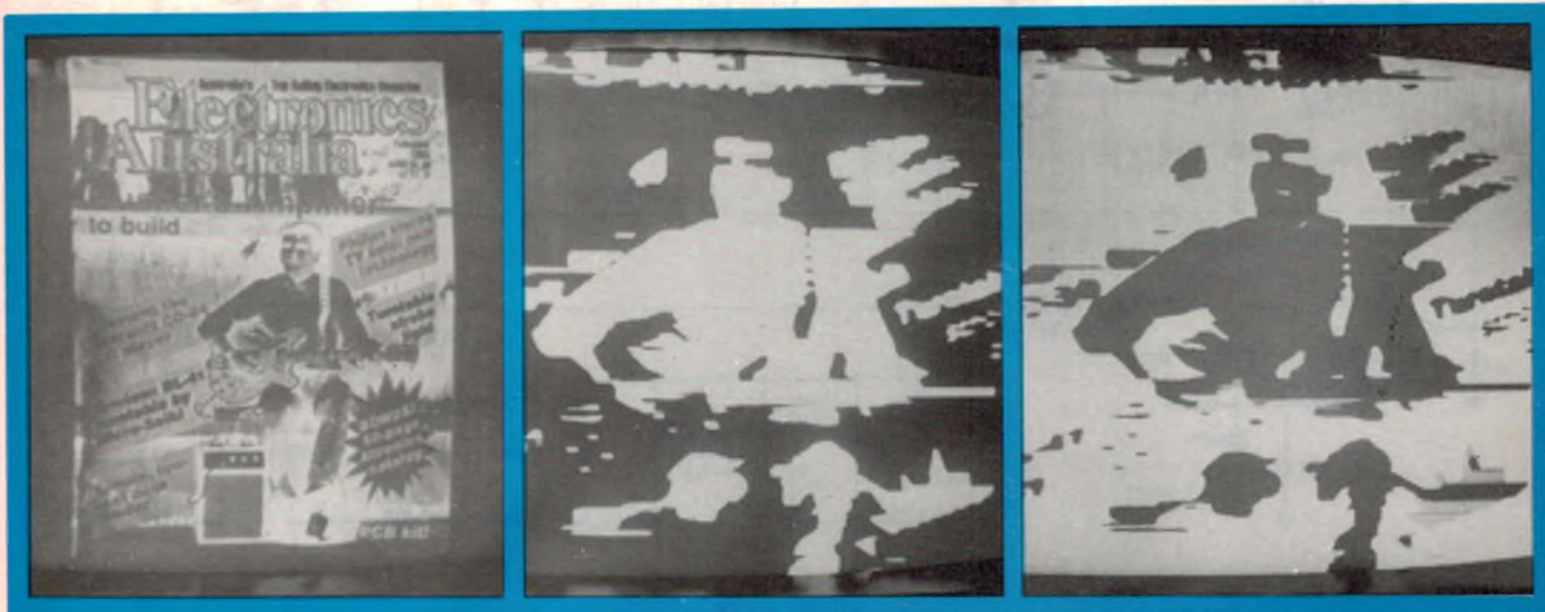
These views show the following special effects: inverted mode, lithographic (discrete) picture, and inverted lithographic picture.
