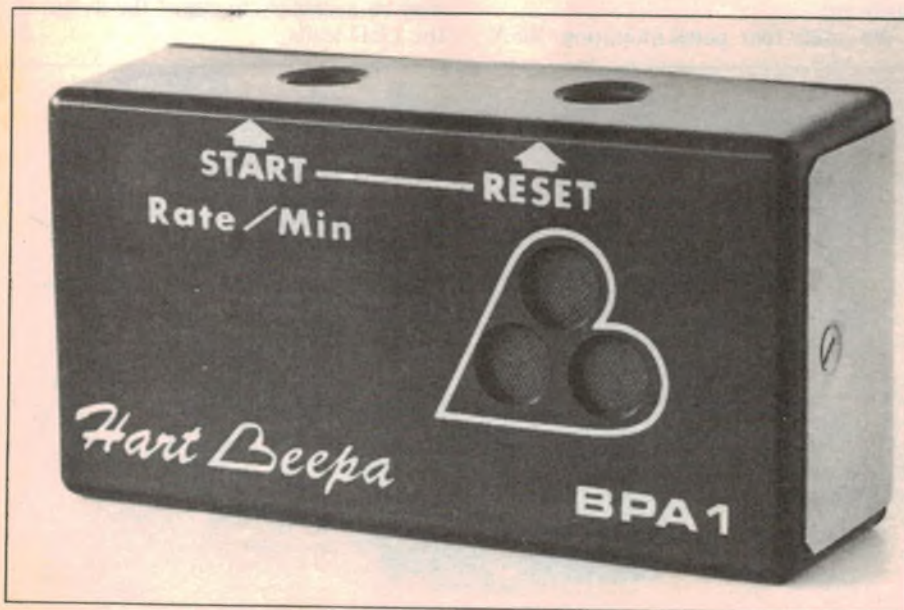
The Hart Beepa is housed in a plastic case with silk-screened lettering.
