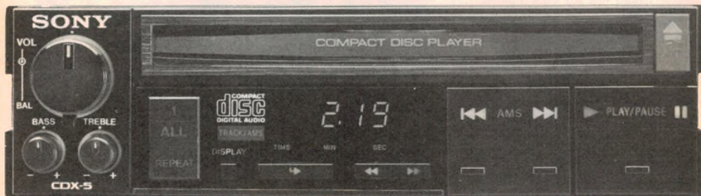
This is an actual-size view of the front panel of the CDX-5. Note the push-in Bass and Treble controls.
