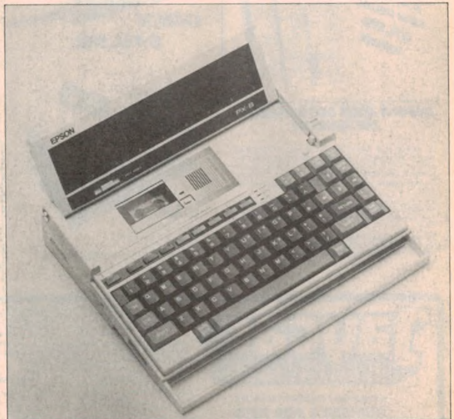
This photograph shows the review model of the Epson PX-8. Note the built-in micro cassette drive and the flip-up display panel.
