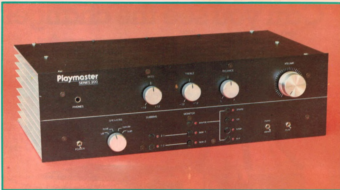
The completed prototype. Most kit versions will be supplied with black anodised heatsinks and black control knobs.
