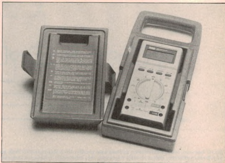
This photograph shows the Fluke model 27, 3½-digit multimeter in the hard carrying case.
