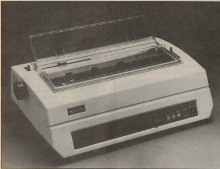
The Daisywheel printer offers a wide range of features, including subscript and superscript commands, bold or shadow printing and underlining. It is good value for money.
