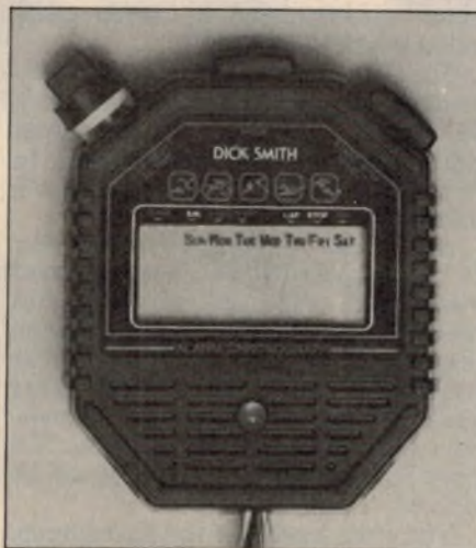
View showing the stopwatch with the modified Reset switch and race in progress LED.
