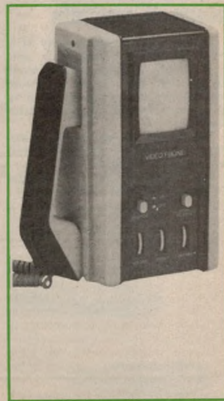
The control centre features a 10cm screen.
