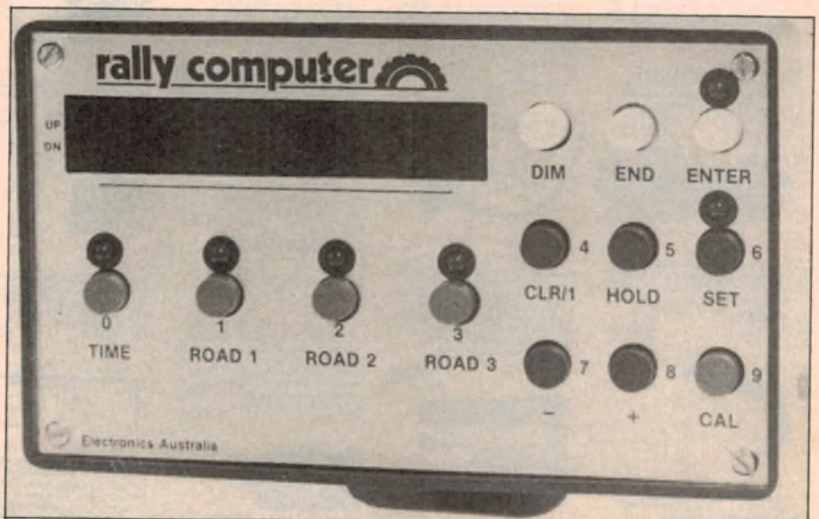
This photograph shows the completed display unit. The socket for the remote pushbutton is on the right-hand side of the case.
