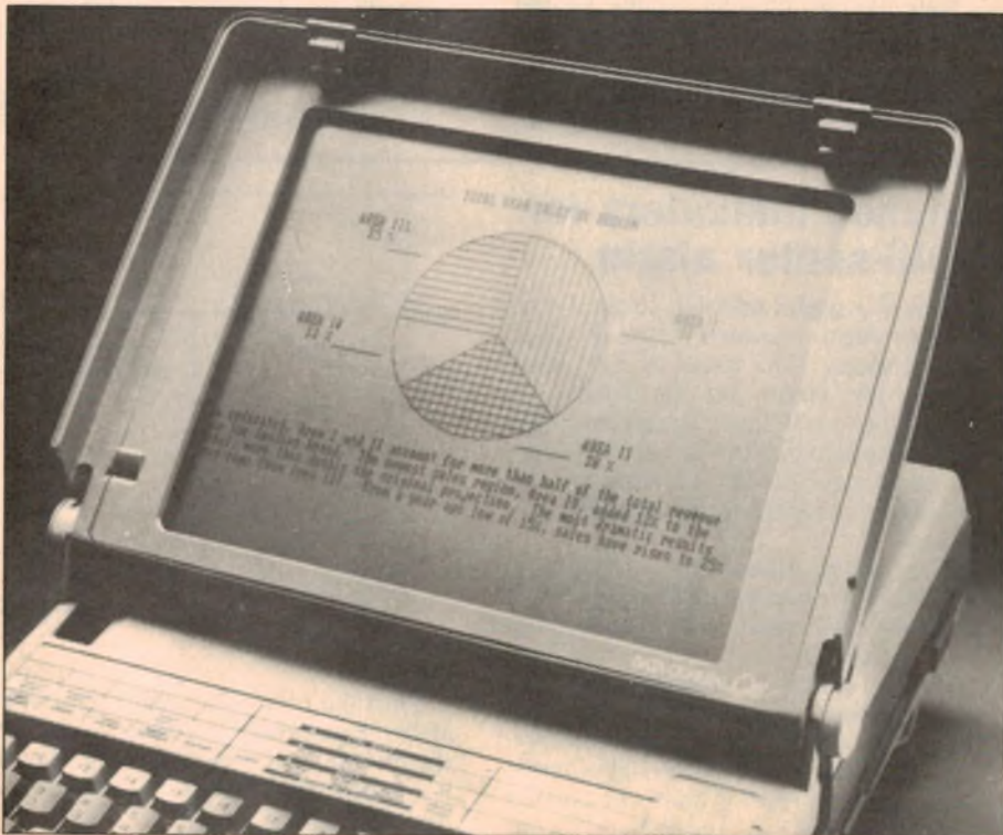
Above: The LCD screen and tilt control of the Data General One.
