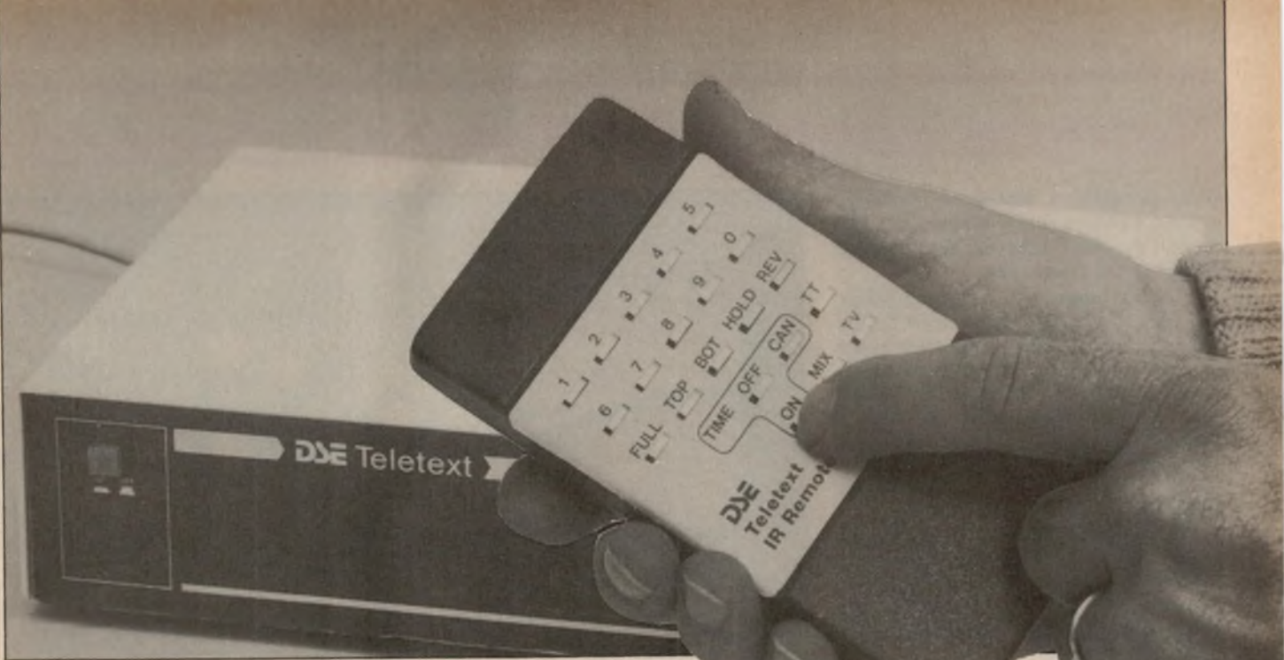
Shown here with the Teletext Decoder, the new infrared remote control duplicates the functions of the original wired unit. Note cutout in the front panel of the main unit, below the mains switch.
