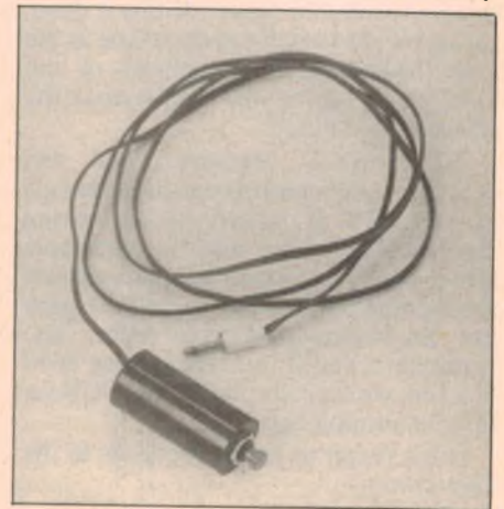
We mounted the remote CLR/1 switch in a discarded plastic film container.
