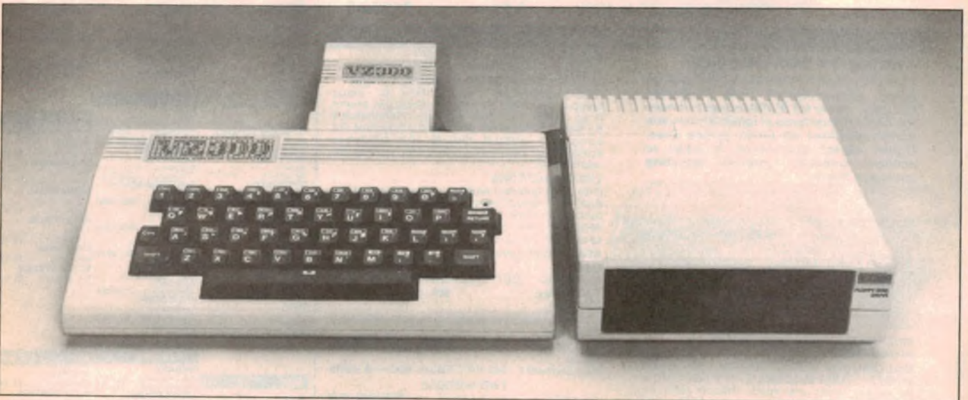
The VZ300 Computer with the DOS (disk operating system) cartridge plugged in at the rear. It, in turn, has a "piggyback" socket for RAM or ROM modules. On the right is the VZ300 Floppy Disk Drive.
