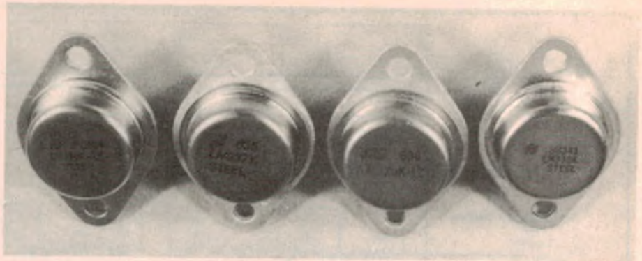
Fig. 2(b): a selection of integrated circuit voltage regulators in standard TO-3 metal cases for easy mounting on heatsinks. Left to right: LM340K-12 (+12V fixed); LM337 K (-1.2V to -37V variable); LM320K-12 (-12V fixed); LM338K (+1.2V to 32V variable).
