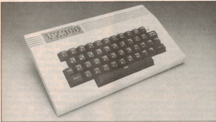
The VZ300 is slightly larger overall than the earlier model but has a much better keyboard with normal space bar.
