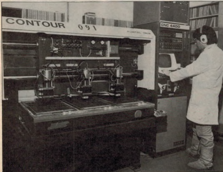
It looks like a drilling machine but it is a numerically controlled high-speed routing machine for cutting the boards to final shape. Ear protectors are a must!
