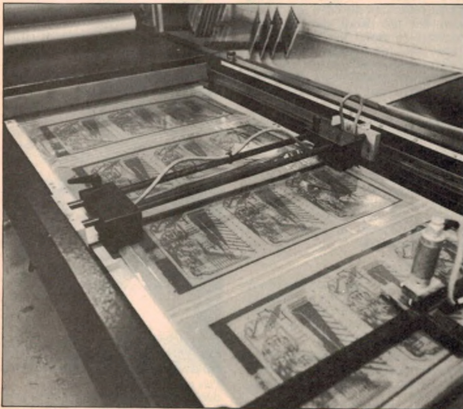
This is one of the later steps in board production: application of dry film solder resist. The film is exposed and developed and then cured by an ultraviolet light and baking process, after which it is solder dipped and levelled.
