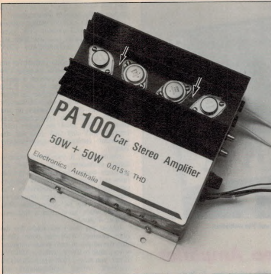
The two arrows indicate the locations of the Vbe multiplier transistors (Q13 and Q24).
