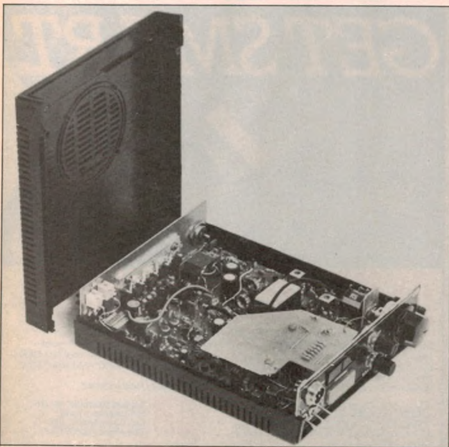
The new transceiver is housed in a compact plastic case.
