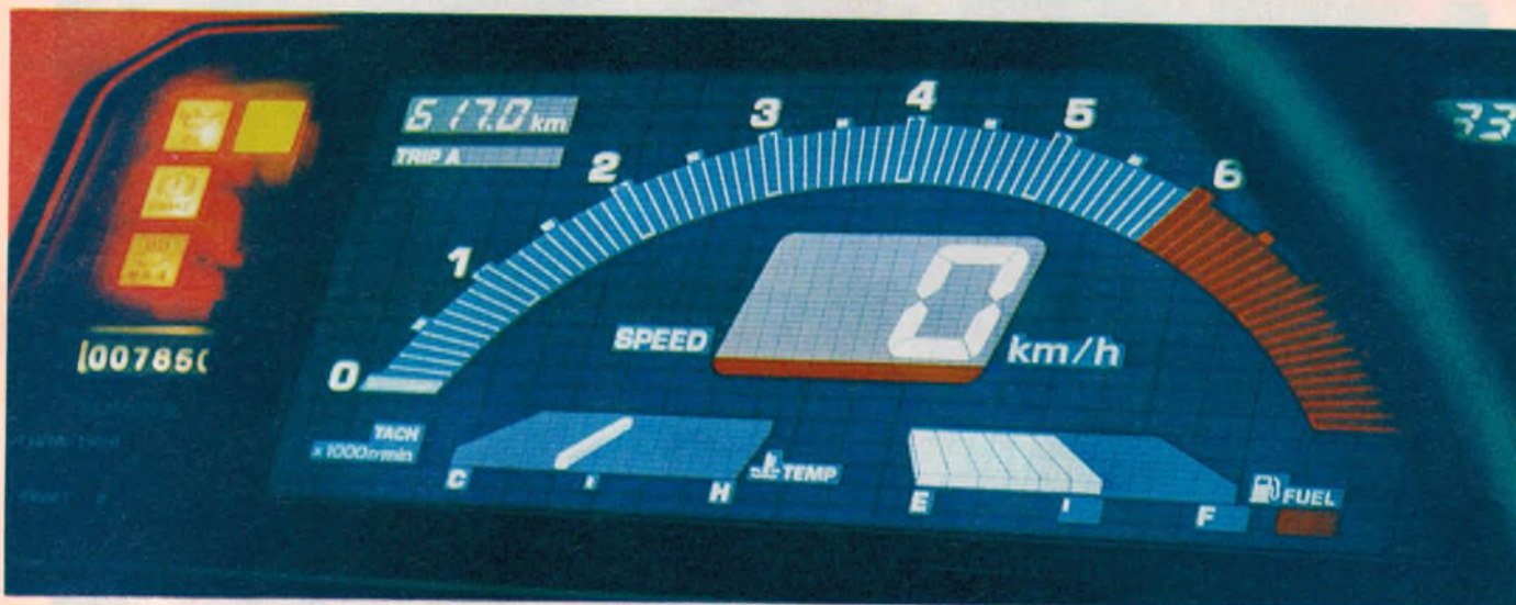
A guest-host liquid crystal display as used by Toyota Motor Corporation. (Photo by courtesy of Soanar Electronics Pty Ltd.)
