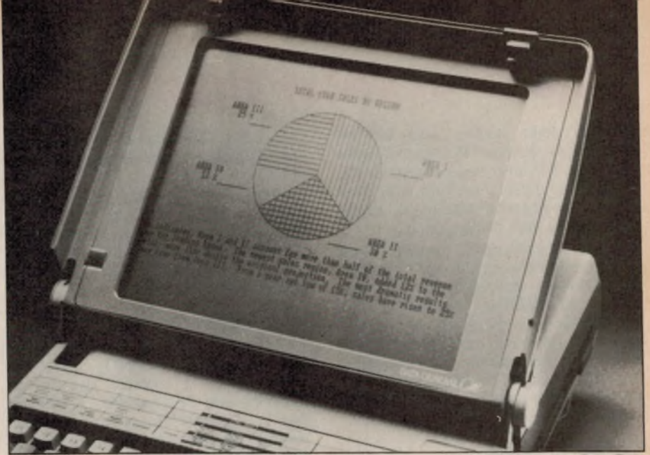
One of the largest multiplexed LCDs presently in commercial use, this is the screen of the Data General One laptop computer.
