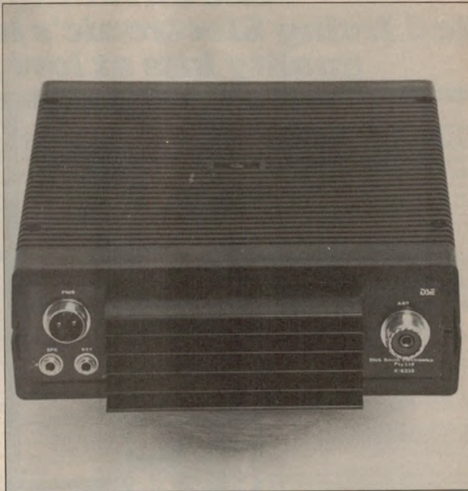
The rear panel carries sockets for power, speaker, key and antenna, together with a hefty heatsink for the transmitter output.
