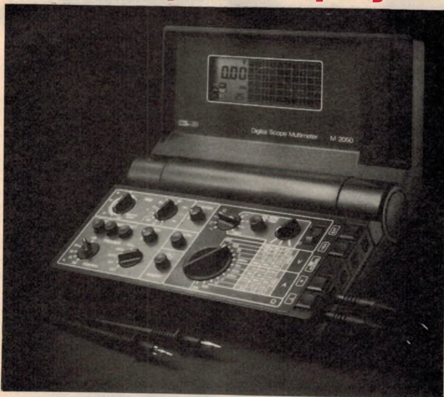
Two separate liquid crystal displays are employed in this BBC Metrawatt/Goerz scope/multimeter. The scope display is a 128 x 64 dot matrix type. (Photo by courtesy of Kent Instruments Pty Ltd.)
