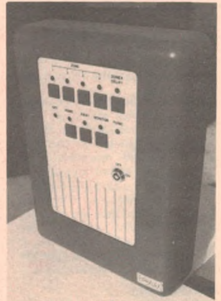
Figure 17. Every manufacturer has a different approach to Control Units. This unit can control 4 separate zones with a time delay in one of them and features an auxiliary siren in the unit.
