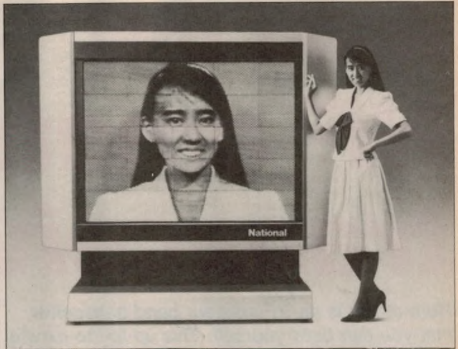
This large screen TV consists of 25 LCD dot matrix panels.
