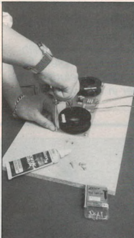
Apply a small amount of white sealant to the rear of the crossover PCB before securing it to the rear panel with self-tapping screws.
