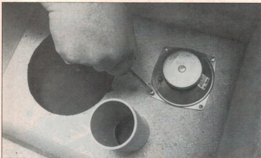
The tweeter is mounted on the inside of the baffle using four 12mm self-tapping screws.
