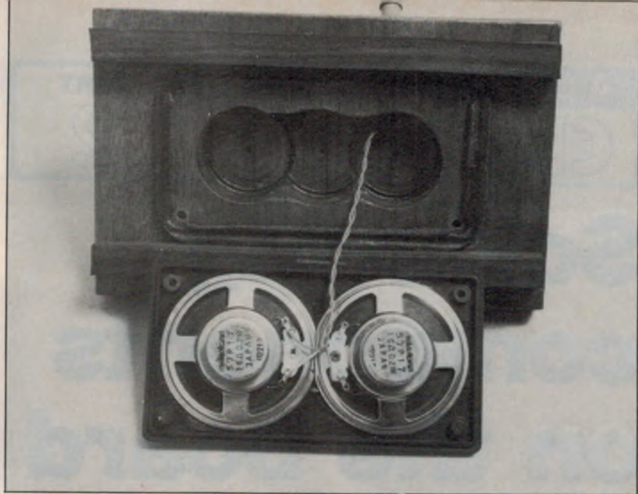
A foam rubber gasket is fitted between the loudspeaker grille and the wooden base.
