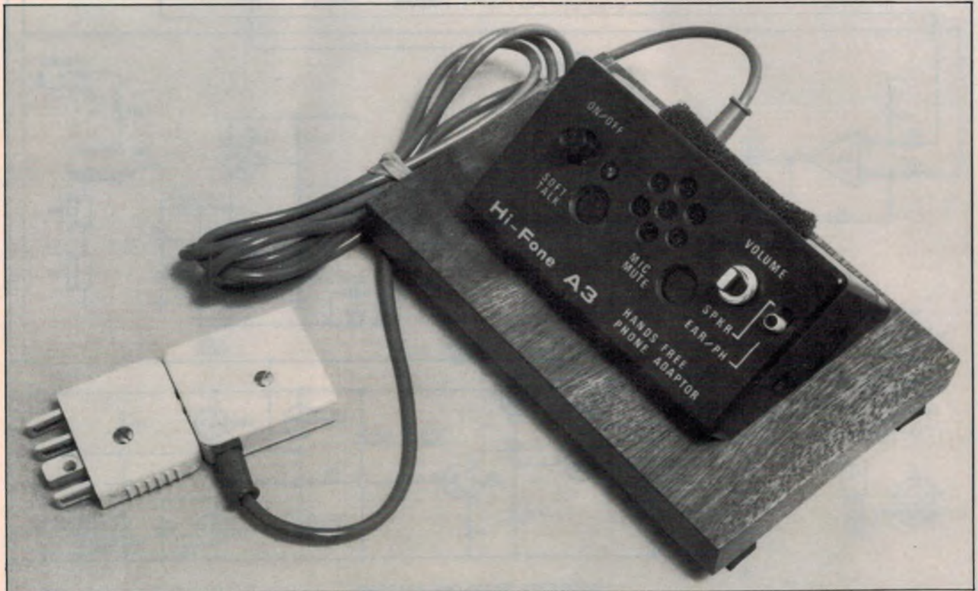
The Hi-Fone is mounted on a solid wooden base which provides good acoustic isolation between the microphone insert in the case and the speakers in the base. Note the modified telephone plug.
