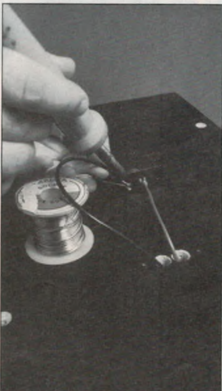
Solder the input leads then apply sealant to the terminal panel before screwing it into position.
