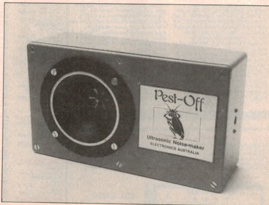
The Pest-Off is housed in a plastic project box and uses a piezoelectric tweeter.
