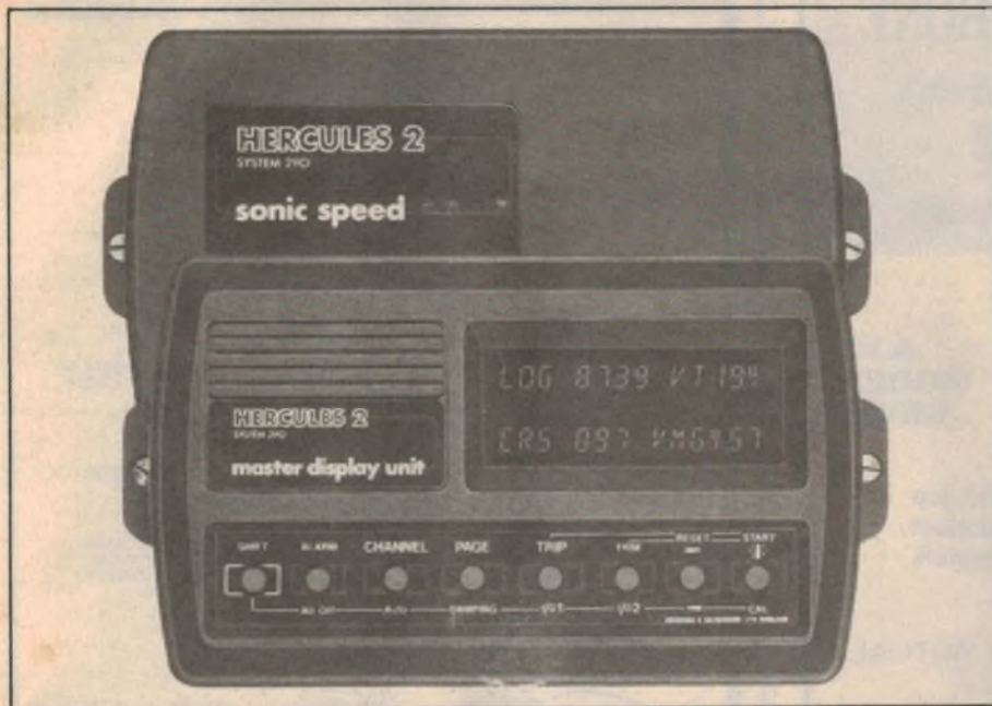
B&G's versatile Hercules 2 system drives a mixture of digital and analog indicators.
