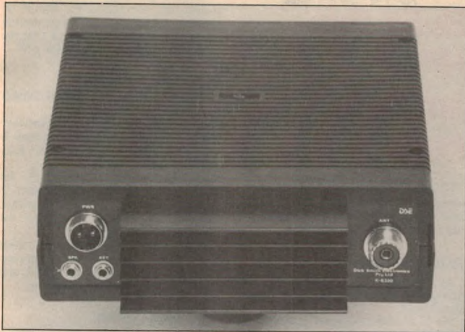
The rear panel carries various sockets for power, speaker, key and antenna connections.
