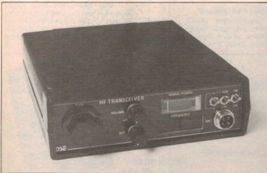
The transceiver is built into an ABS plastic case with two interlocking halves.
