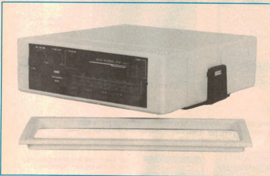
Marine entertainment equipment must be specially designed to prevent corrosion. Both the GME GR926 (above) and GR934 radio-cassette players feature plastic cases, heavy-duty plating and moisture resistant coatings on circuit boards.
