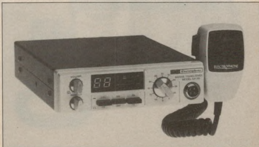
The GME GX281 is a popular 27MHz marine transceiver. It sells for about $150.
