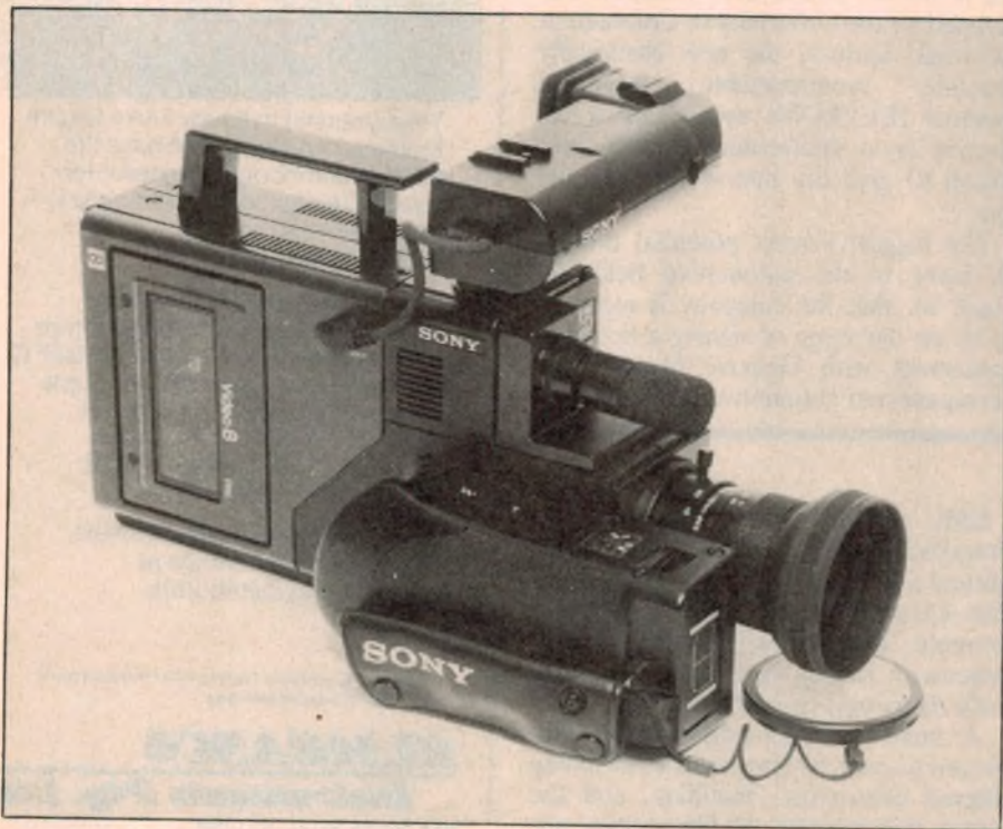
From the front, the CCD-V8 looks much like any other modern domestic video camera, except that it is completely self-contained. Unlike Betamovie, it contains full in-built playback facilities.
