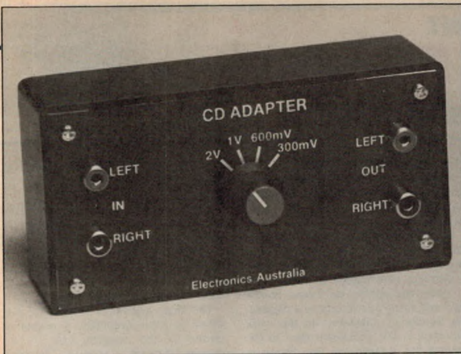
The circuit is built into a low-cost plastic case.
