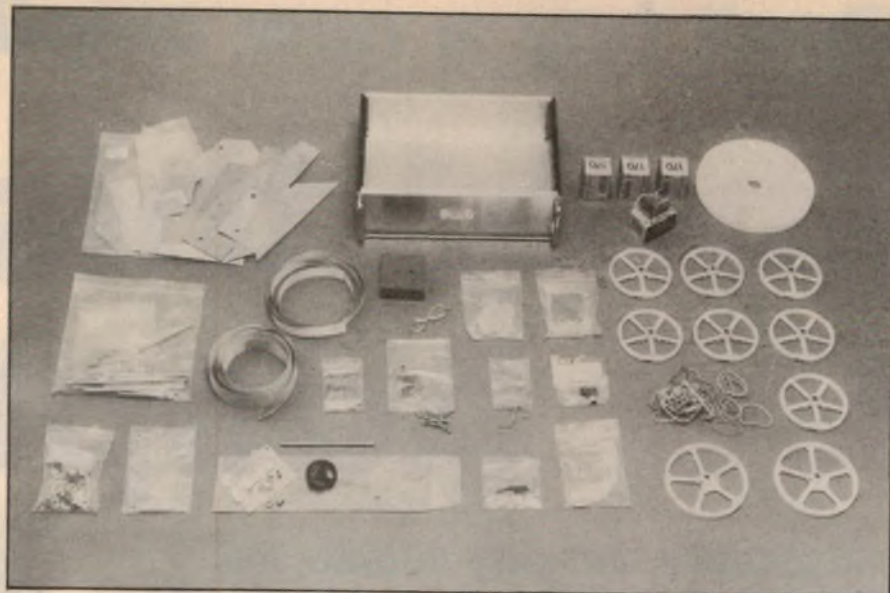
Algernon consists of PCB laminate, dial drums, rubber bands and electric motors.
