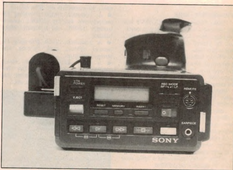
When placed flat on a shelf or in its adaptor tray for playback &c, the CCD-V8 takes on the appearance of a portable deck, with the usual array of user controls. Add a timer/tuner and it becomes a complete VCR.
