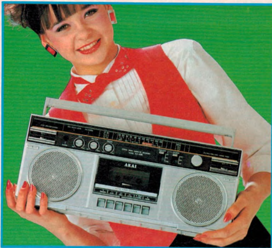
Beloved of teenagers and others who like to have a radio around, this Akai AM/FM stereo cassette-radio typifies dozens of similar models. Portable, versatile and adequate for casual listening, they nevertheless fall well short of hifi standards.
