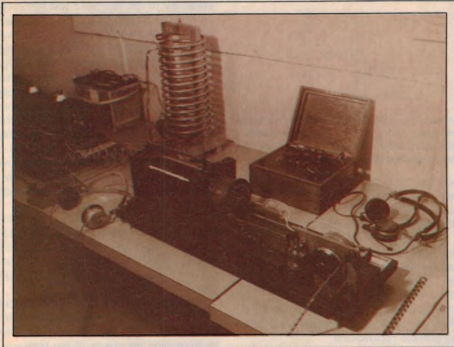
The companion receiver uses a loose coupler and a cat's whisker detector.
