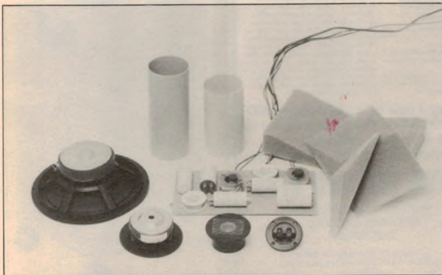
The crossover network uses large metallised polypropylene capacitors.
