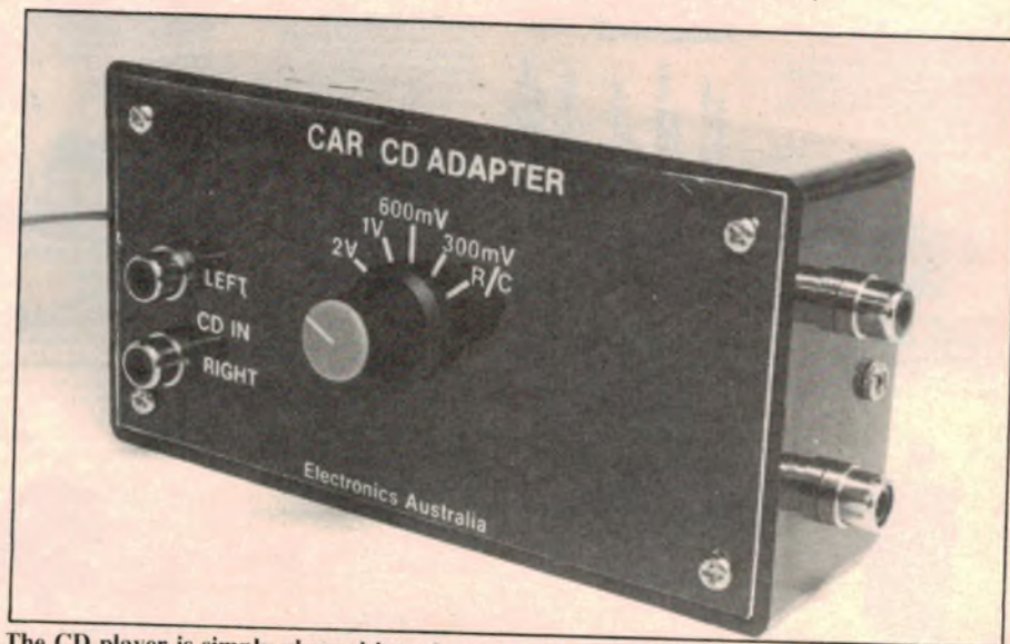
The CD player is simply plugged into the two front-panel RCA sockets.
