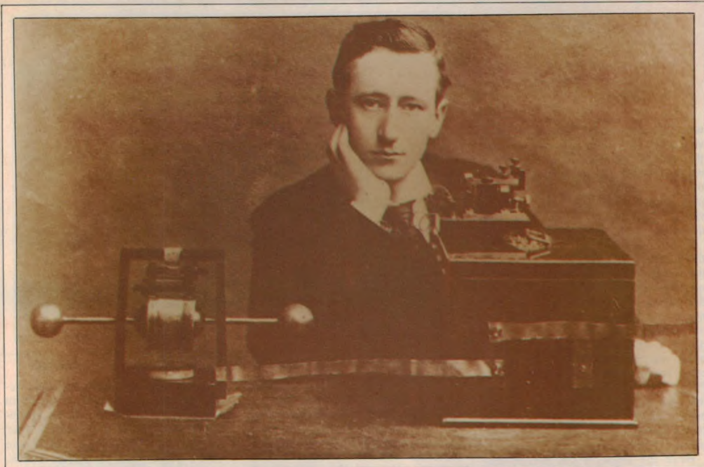
Guglielmo Marconi with his experimental wireless apparatus of 1897. The black box contained the spark transmitter.
