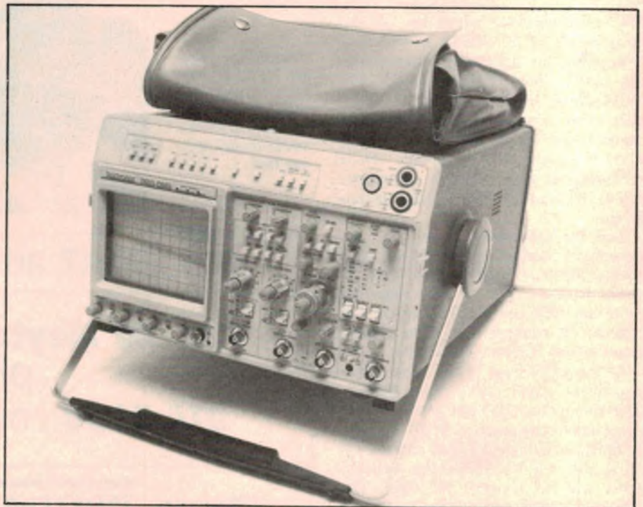
Many of the controls for the 2465 have more than one function. The digital multimeter controls are on the upper panel.
