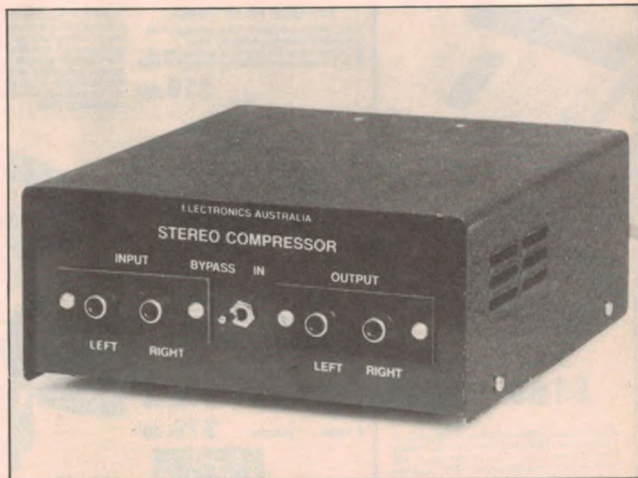
The input and output RCA sockets are mounted on the front panel of the metal case.
