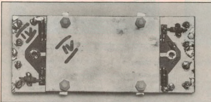
Above: this view shows the completed microstripline PCB with the cover plate attached.
