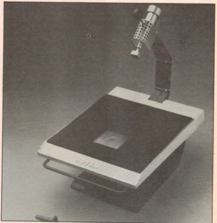
Fig.17: This Royel position table has a special hollow head to heat up the SMD to be removed and a vacuum feed to lift the device off the board.
