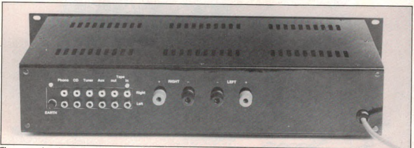
The rear panel carries the RCA input sockets and the loudspeaker terminals. Make sure that the mains cord is securely clamped.
