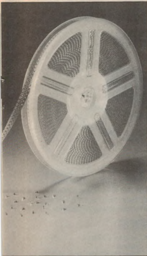
Fig.3: Surface mount devices can be used alone or mixed with other components and be mounted on or below PC boards. (Diagram by courtesy of Siemens.)
