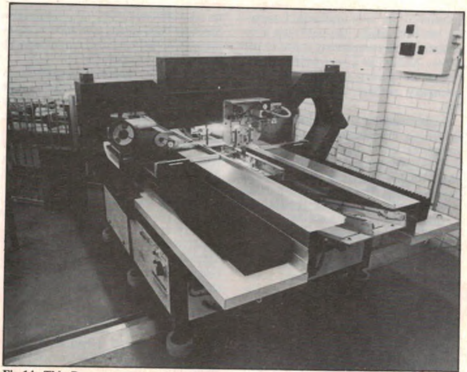
Fig.14: This Dynapert NPS 500 pick-and-place machine can accept up to 120 different component feeds and place 6500 devices per hour. The machine is installed at Appliance Control Systems, Revesby, NSW.
