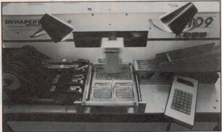
Fig.19: This photo shows the rapid action of a pick-and-place machine as it grabs components from the tapes and places them on the boards. (Yellow Light.)
