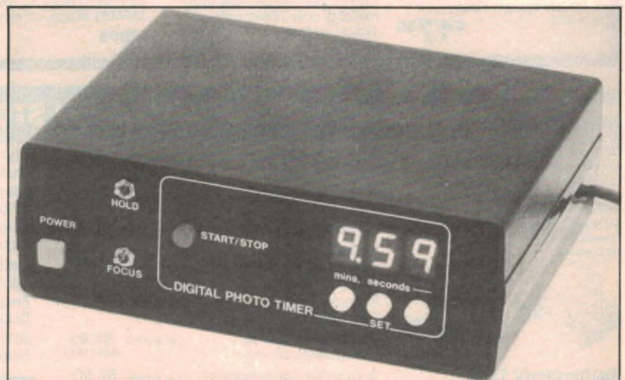
The new Digital Photo Timer is housed in a standard plastic instrument case.
