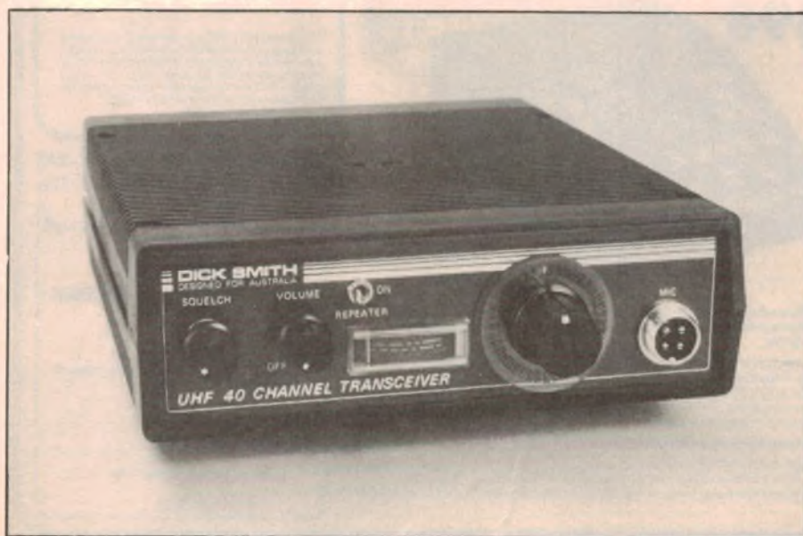
The Explorer UHF amateur transceiver originally covered 40 channels from 438.025 to 439.000MHz.
