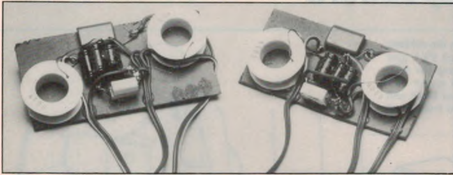
The crossover networks are relatively simple and are supplied preassembled.
