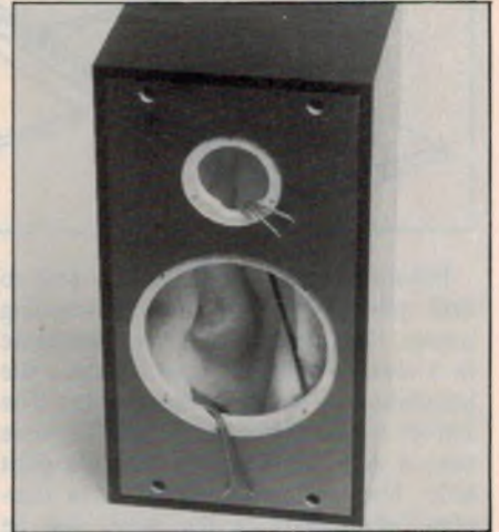
This view shows the assembled cabinet, prior to mounting the loudspeakers.
