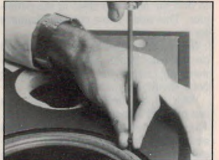
Take care when mounting the drivers — it's all too easy to punch a hole through a cone.
