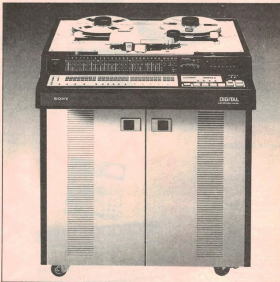
Now available in Australia, Sony's PCM-3324 is the first of a new generation of standardised multi-track, fixed head studio digital recorders, intended to take over from existing analog models.
