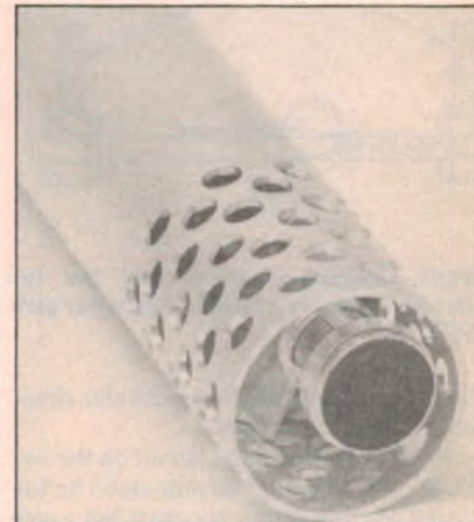
The "business" end of The Microphone. The electret insert is clearly visible.
