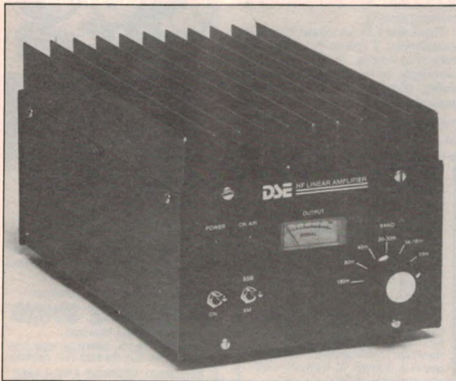
The completed HF linear amplifier —150W PEP and switchable output filters.
