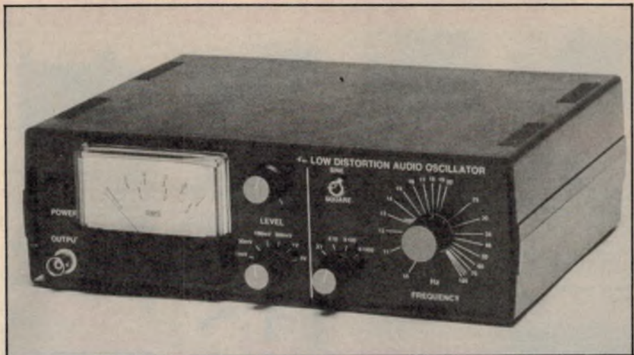
The alternative version features the output level metering circuitry.
