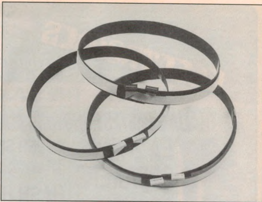
These three loop coils cover the range of frequencies from 200kHz to around 13.5MHz.
