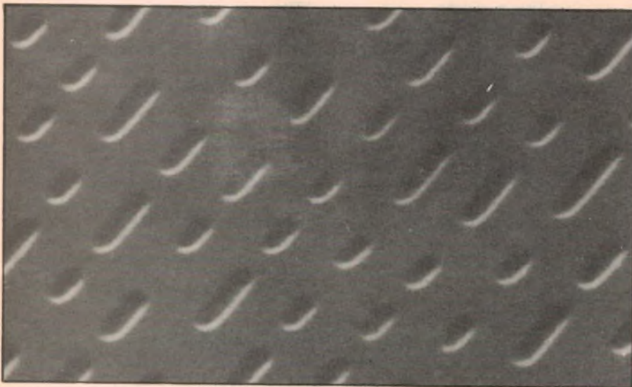
A microphotograph of the pits or bumps in a typical compact disc. It has been calculated that, for the pits to be magnified to rice-grain size, the effective disc diameter would be around 800 metres! (By courtesy of Philips).
