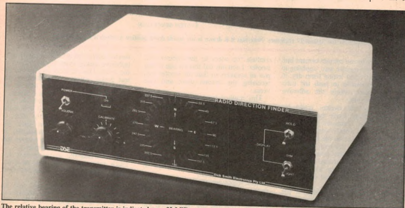
The relative bearing of the transmitter is indicated on a 32-LED compass rose.
