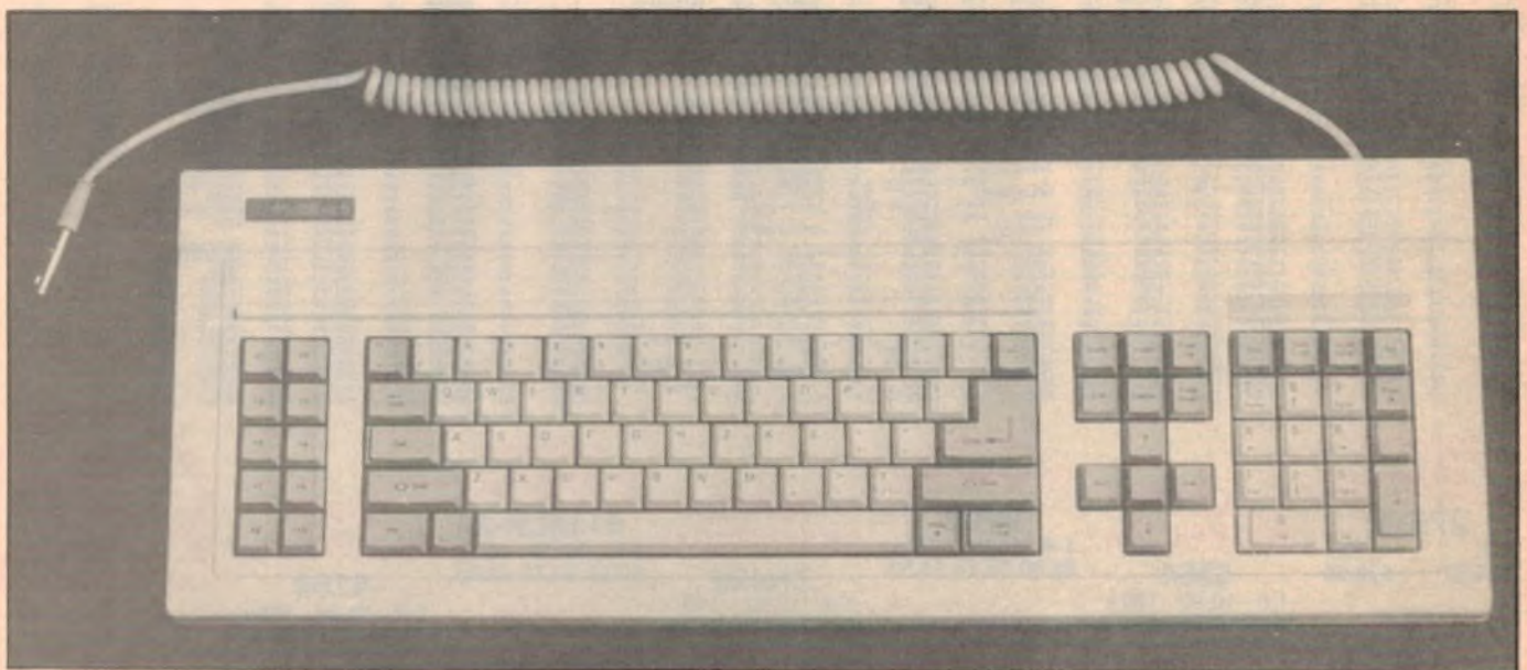
The keyboard of the Multitech PC-700 has much the same features as that of the IBM PC/AT except for the separate cursor keys.
