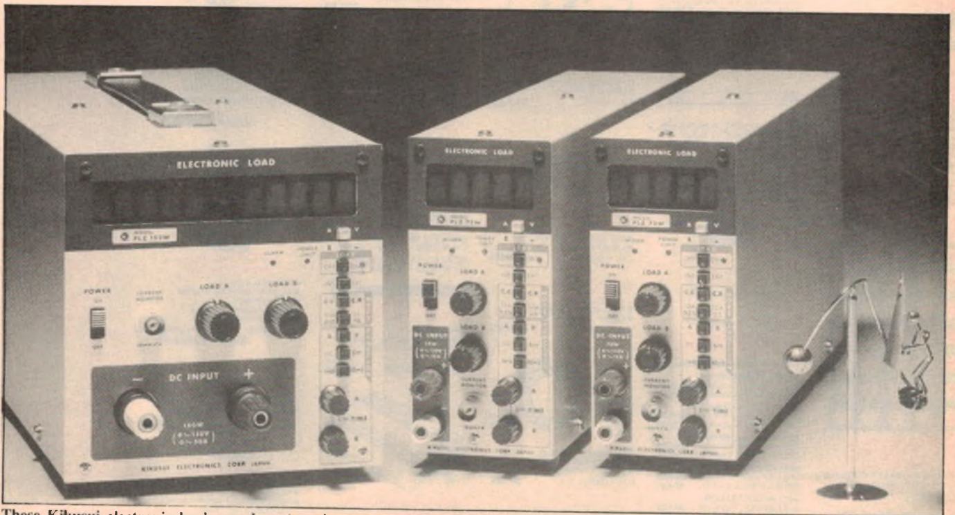
These Kikusui electronic loads can be set to draw any current up to their power ratings of 70 and 150 watts. They are distributed by Emona Pty Ltd.
