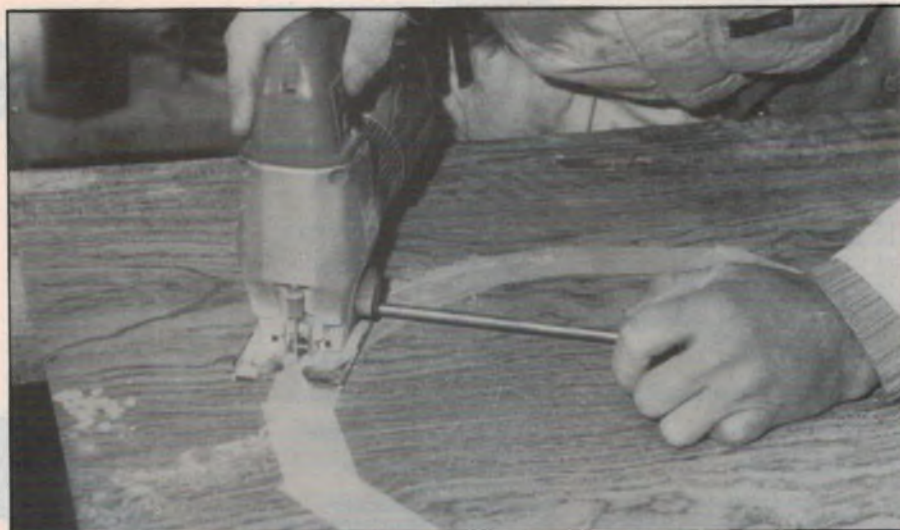
Photo 4: use your jig saw to make the cutout for the loudspeaker. Note use of masking tape to prevent chipping of the veneer.
