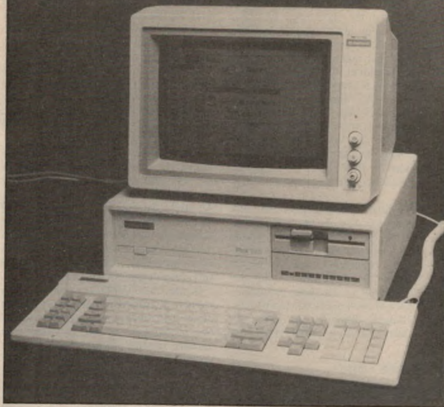
The standard Multitech PC-700 comes with two 360K floppy drives. This machine was fitted with the optional 20M hard disc drive.
