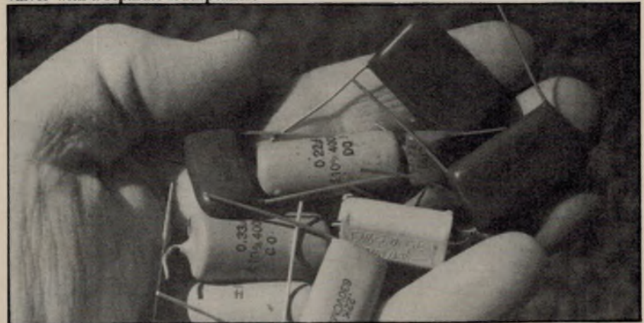
Old paper capacitors should be replaced with high voltage (400-630V) polyester equivalents.
