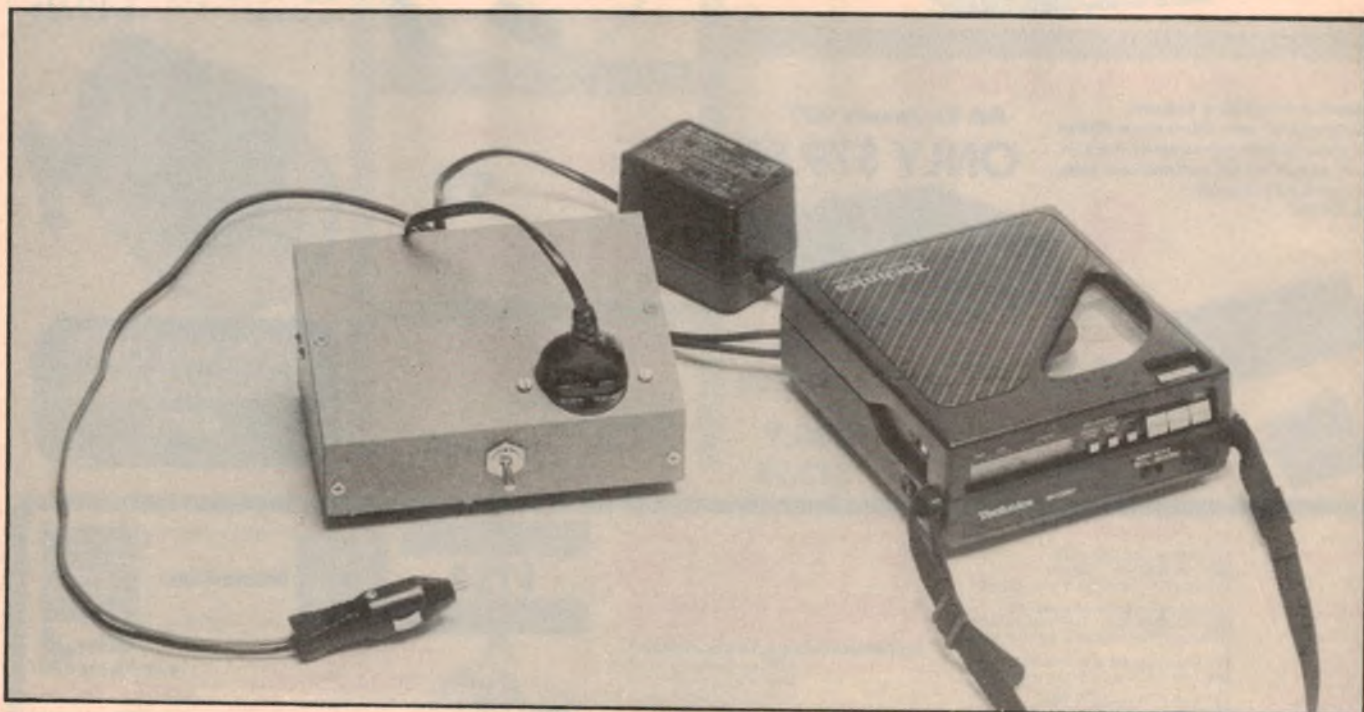
The new inverter can be used to power any portable CD player which has a plugpack adaptor and draws up to 15W.
