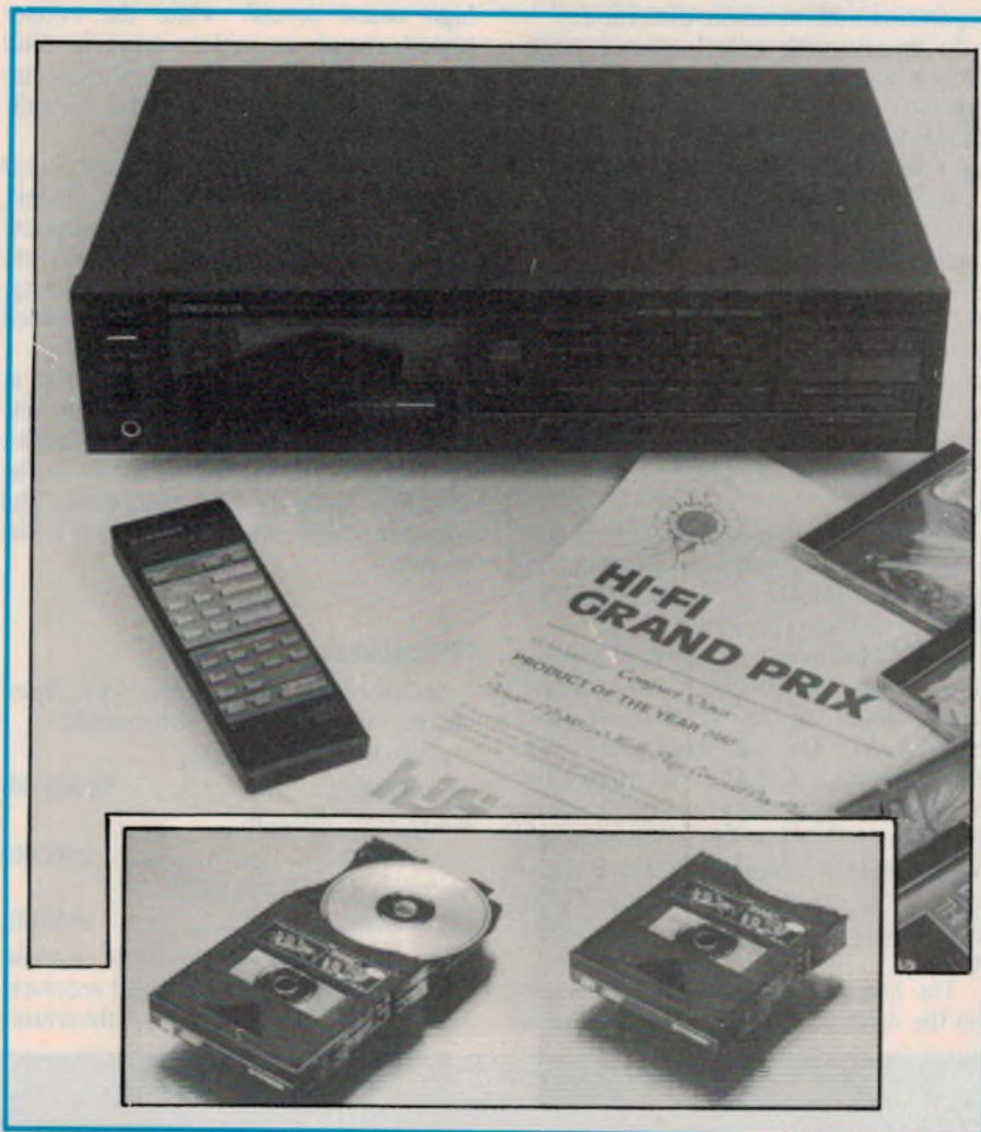
Pioneer's PD-M6 multiplay CD player has a cassette loading system which lets it handle up to six compact discs.
