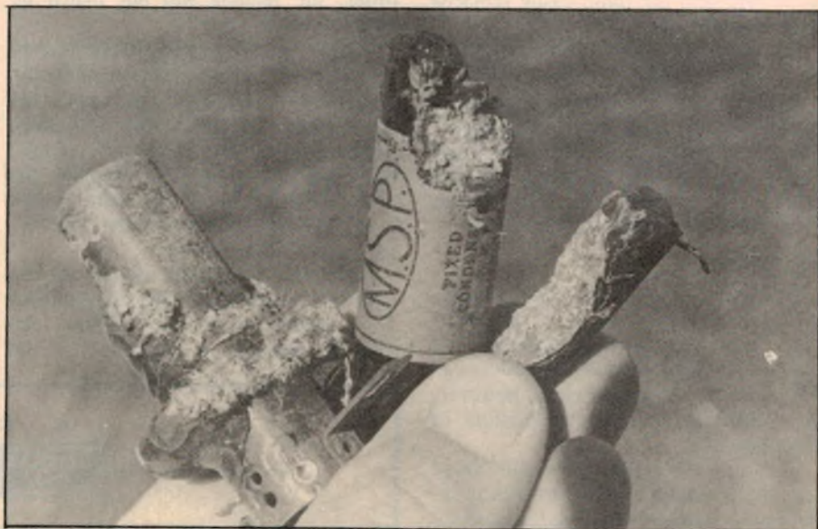
Vermin, namely rats and mice, can do considerable damage to old radio components. A thorough checkout before plugging the set into the mains will detect such hazards.
