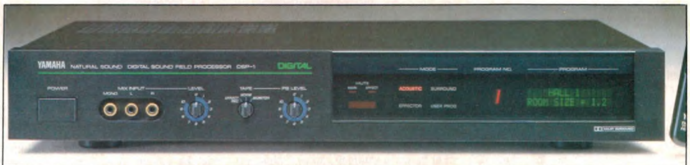
The Yamaha DSP-1 digital signal processor reproduces the acoustic environment of large and small concert venues.
