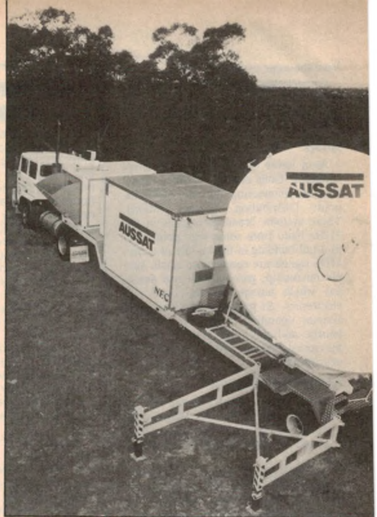
Aussat transportable Earth stations can be towed to virtually any site in Australia. The stations may be used by commercial organisations such as mining companies, or to cover special events.
