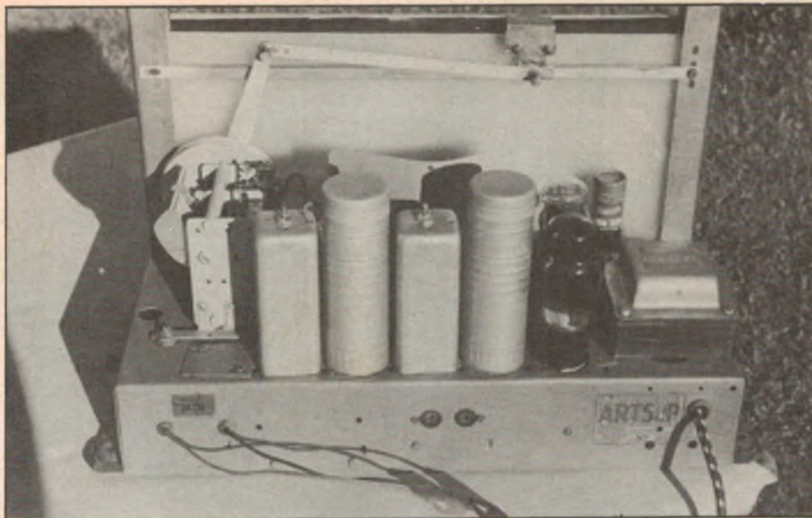
A fully restored radio, ready to go back into the cabinet. Note crank used to move dial pointer.
