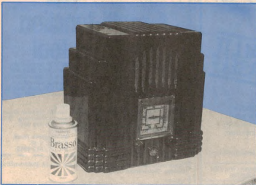
"Brasso" metal polish is ideal for cleaning up old bakelite cabinets such as this mid 1930s Radiola.
