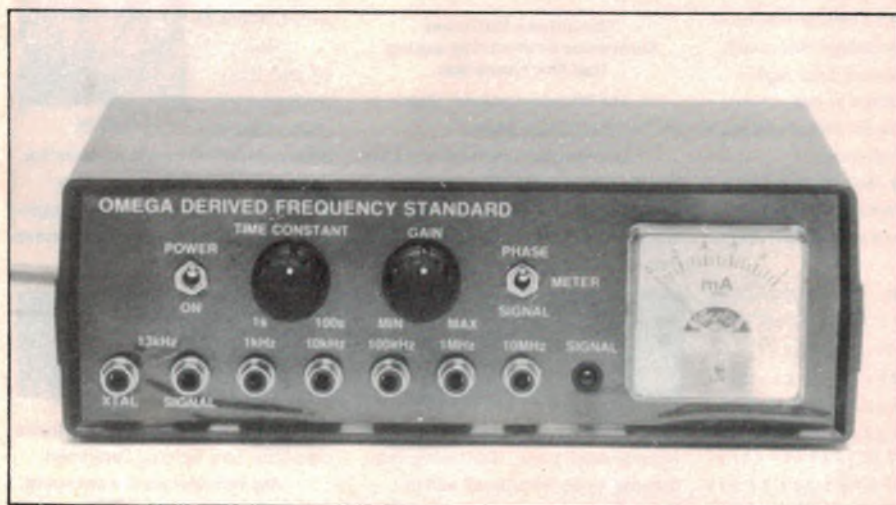
The new frequency standard provides five cesium-locked outputs at 1kHz, 10kHz, 100kHz, 1MHz and 10MHz.
