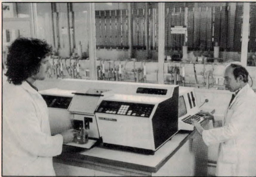
Precise control of chemistry in the etching and plating stages of PCB production is essential. This facility at Teknis Pty Ltd includes an atomic absorption spectrophotometer.
