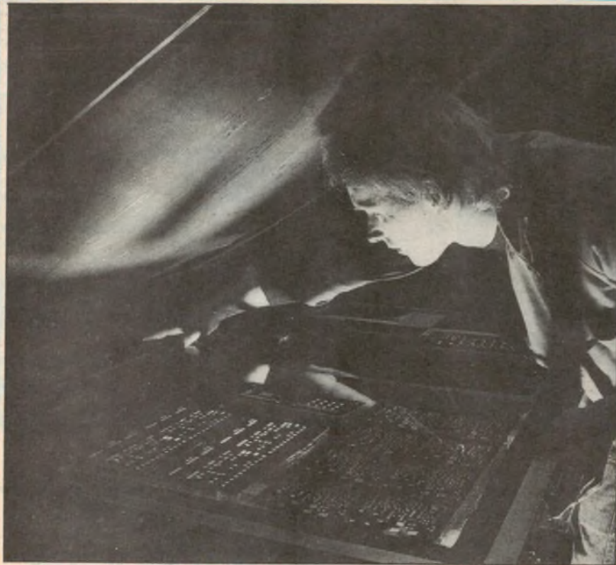
This is a vacuum exposure table where UV light transfers the image of the PC pattern onto the photosensitised copper laminate.
