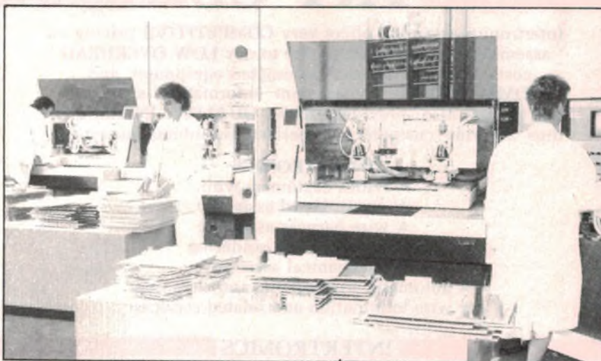
Another big investment for PCB manufacturers involves the numerically controlled high speed drilling machines. Photo courtesy of Teknis Pty Ltd.
