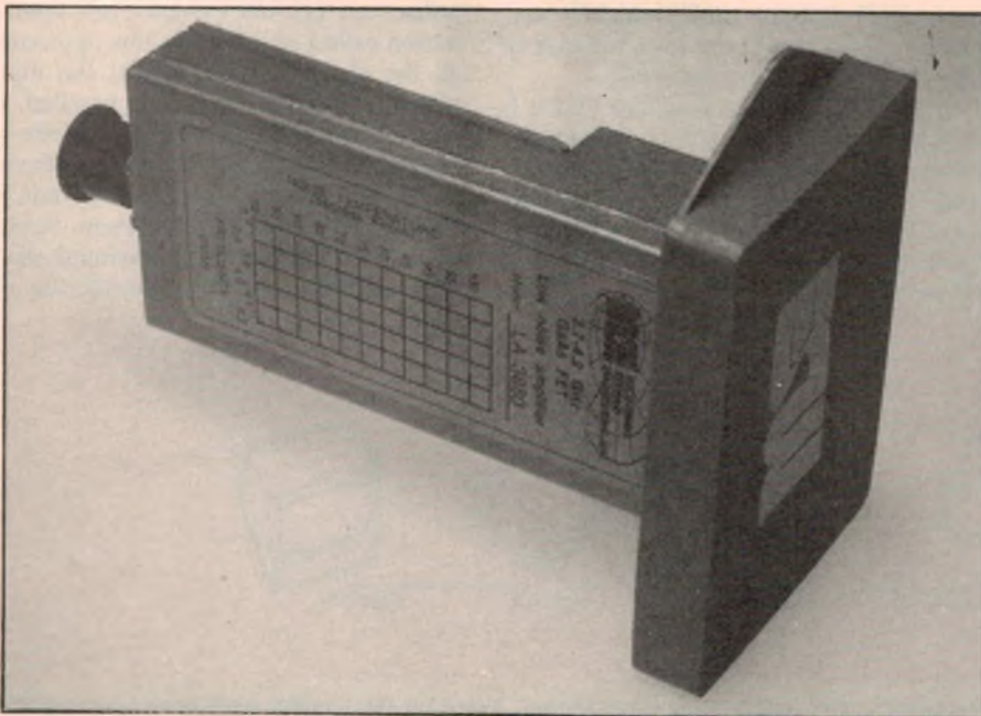
This low noise amplifier (LNA) covers the 4GHz 'C' band of the Intelsats. (Dick Smith Electronics).
