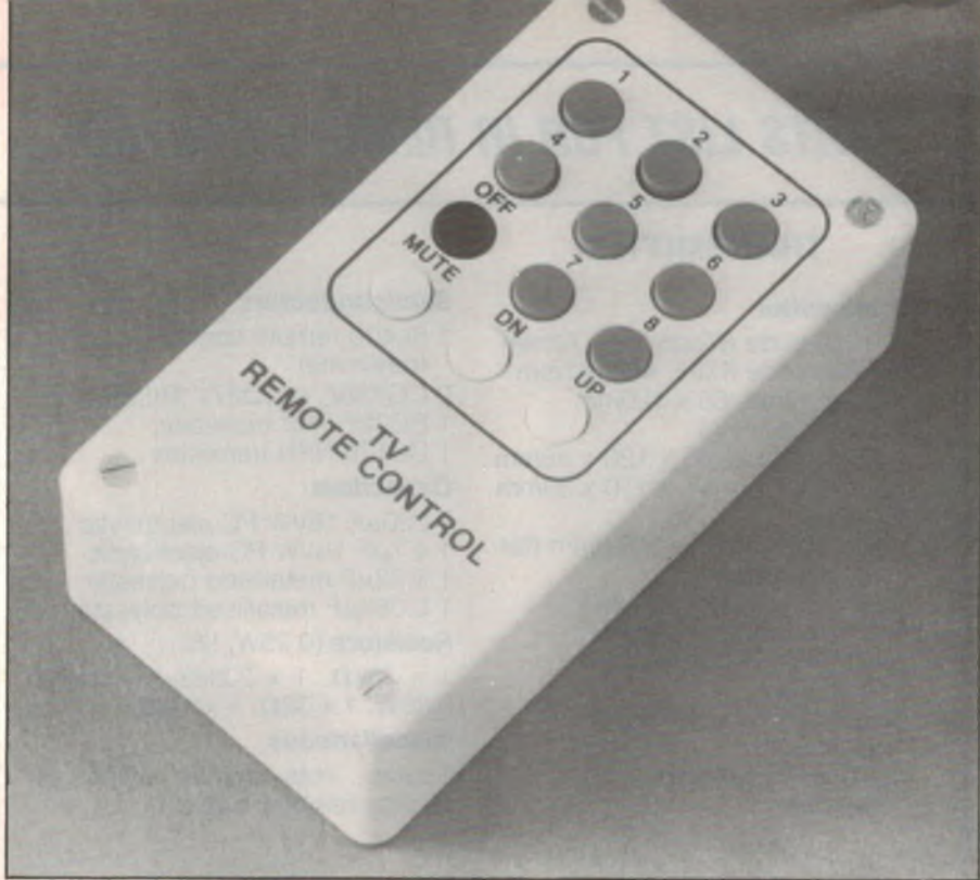
Alternative version of the transmitter, mounted in the larger of the two standard cases. Leave out the buttons for those functions that you don't need.
