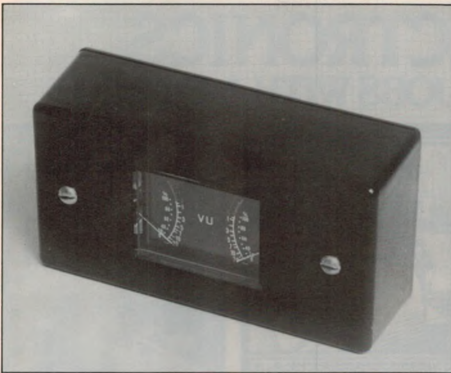
The prototype was housed in a small plastic case. Backlighting for the meter scales is provided by two small 6V lamps mounted on the PCB.
