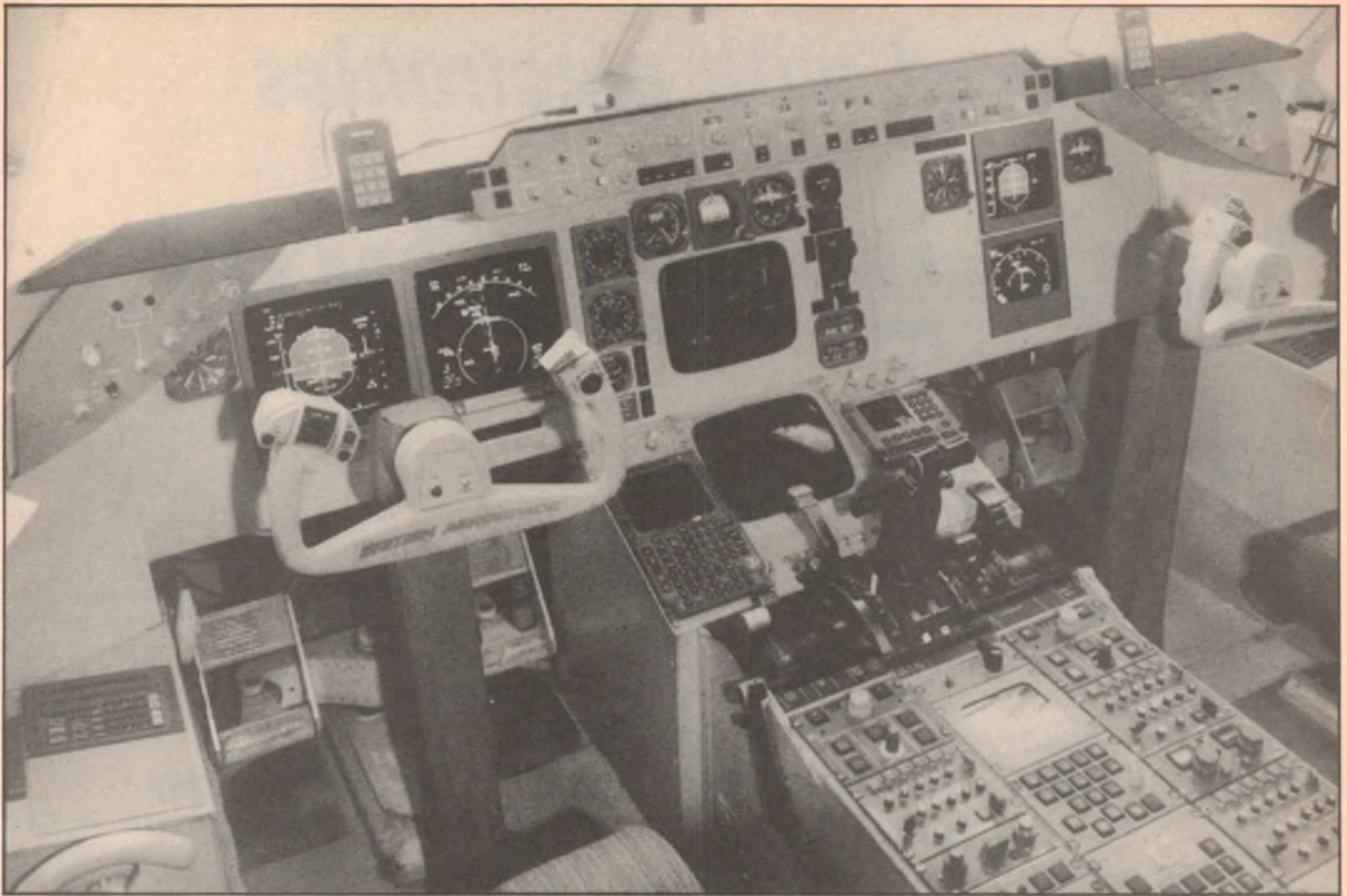
In this mock-up of a future cockpit, computer generated images on cathode ray tubes replace conventional needle gauges. (Photo: British Aerospace).
