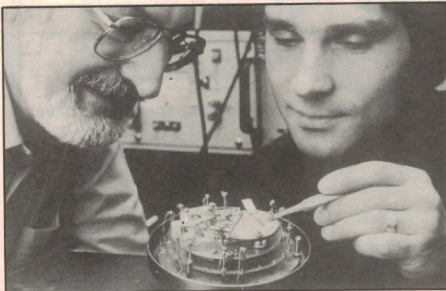
1986 NOBEL PRIZE IN PHYSICS: Heinrich Rohrer (left) and Gerd K. Binnig of the IBM Zurich Research Laboratory adjust a sample in the chamber of an early Scanning Tunneling Microscope (STM). Without the knowledge of materials gained using the STM, a lot of superconductor progress would not have been possible.
