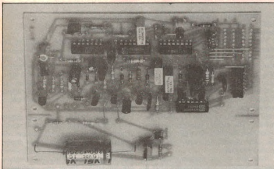
The PC board for the combination lock. Programming for the code digits is carried out using the diodes and links in the top right hand corner.
