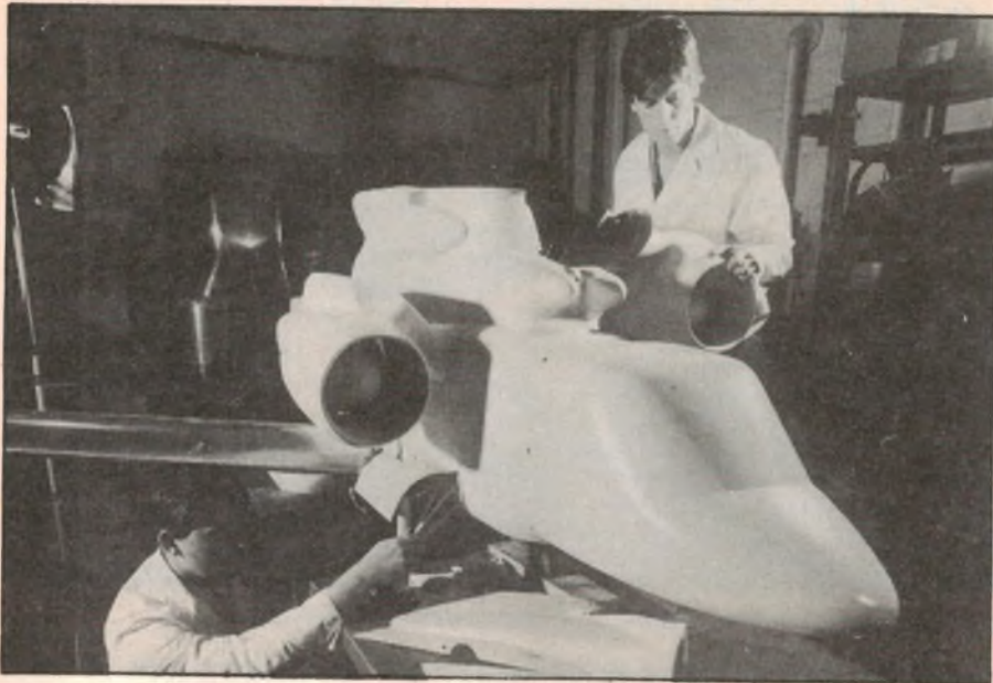
A one-sixth scale model of the Rotor Systems Research Aircraft that will test-fly X-wing, being prepared for wind-tunnel tests.
