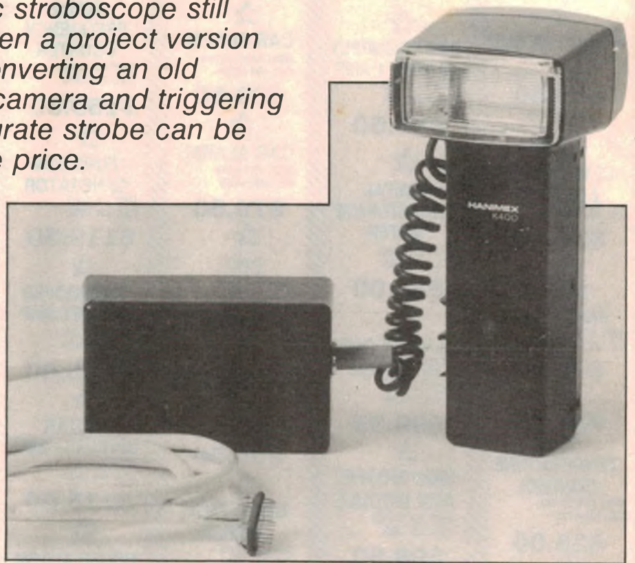
The authors' prototype strobe interface, with a typical low-cost electronic flash. How to modify the flash is explained.
