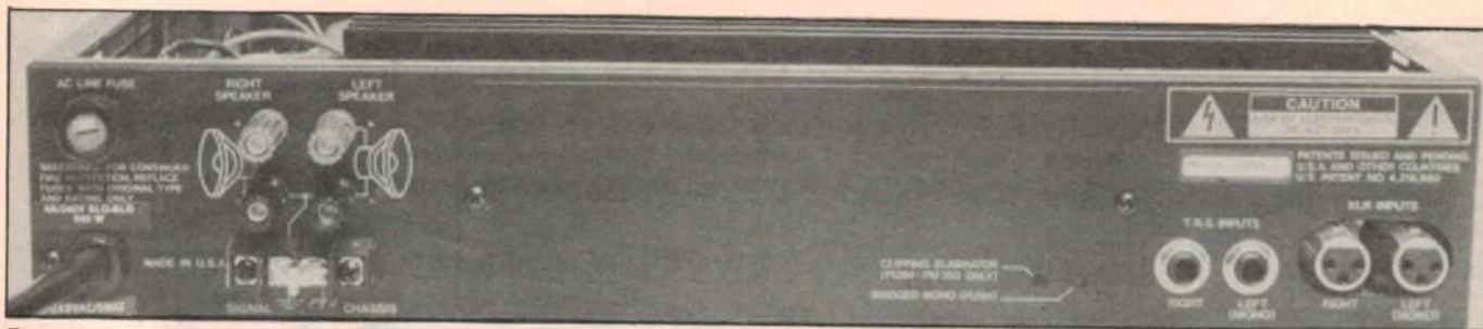
The rear of the PM-350. Both tip-ring-sleeve and XLR input connectors are provided, for both channels. Recessed switches are used for bridged-mode mono and clipping elimination.
