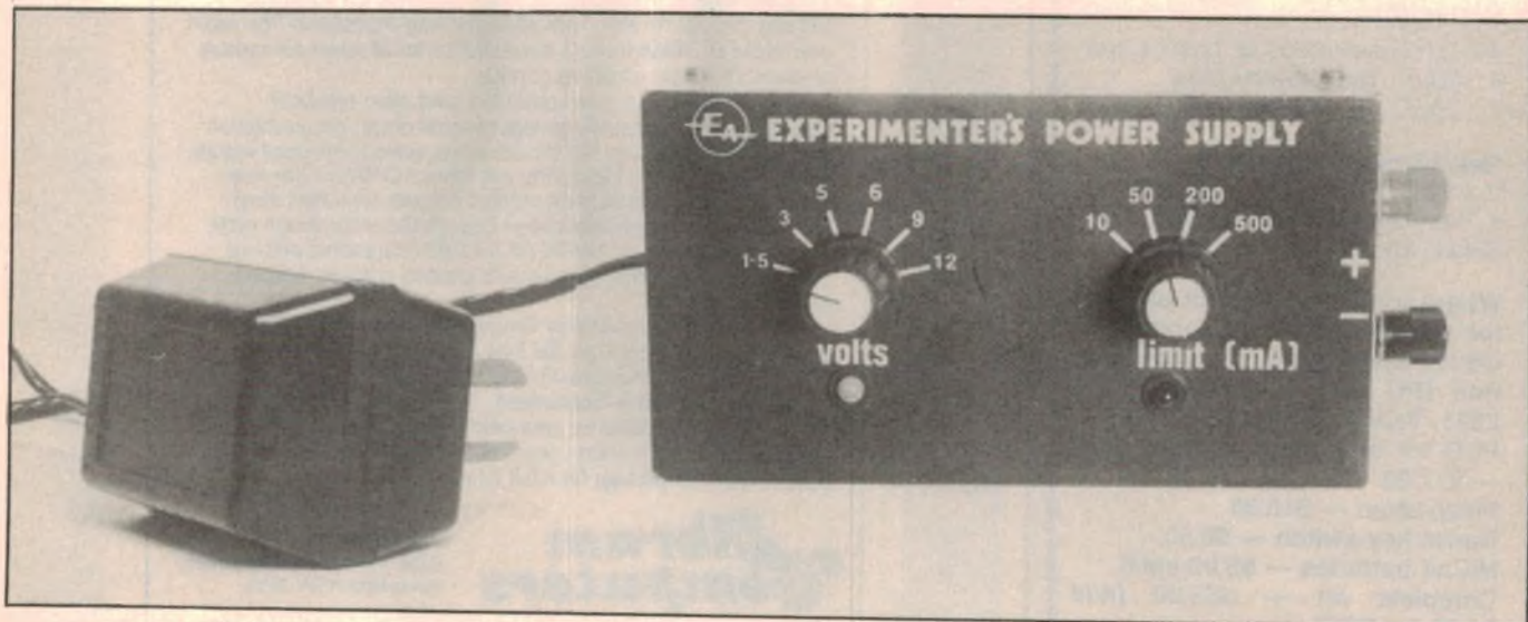
The supply is built into a low cost aluminium case. An AC plug pack provides total isolation from the mains.
