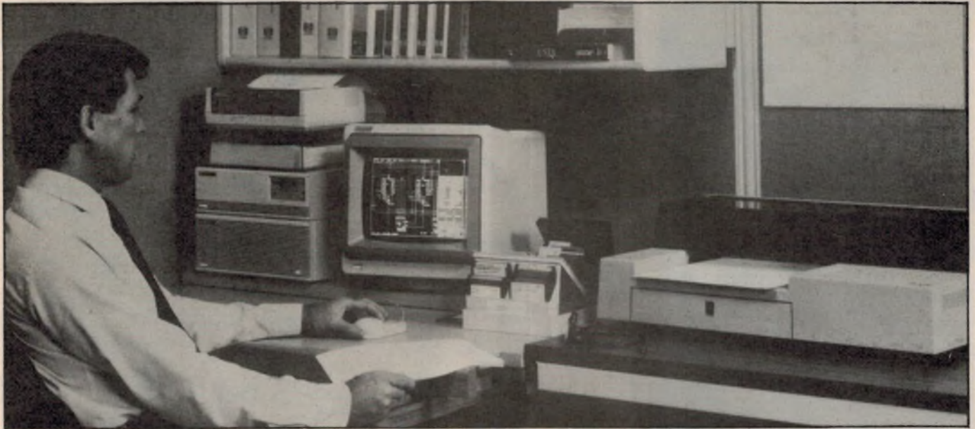
The Hewlett-Packard HP 9000 series 300 workstation, being used for schematic circuit capture. (Courtesy Hewlett-Packard Australia)
