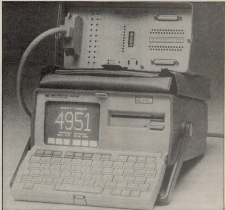
Hewlett-Packard's HP 4951C set up ready for action, with its main menu screen visible. All functions are easily selected using menus and the six function keys just below the screen.
