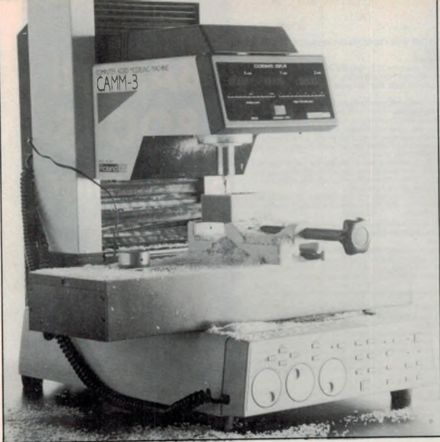
This new computer-aided modelling machine from Roland Corporation hooks up to a PC-based CAD system and will automatically machine a prototype from wax, plastic, wood or light metal. Further details are available from Roland on (03) 241 1254.
