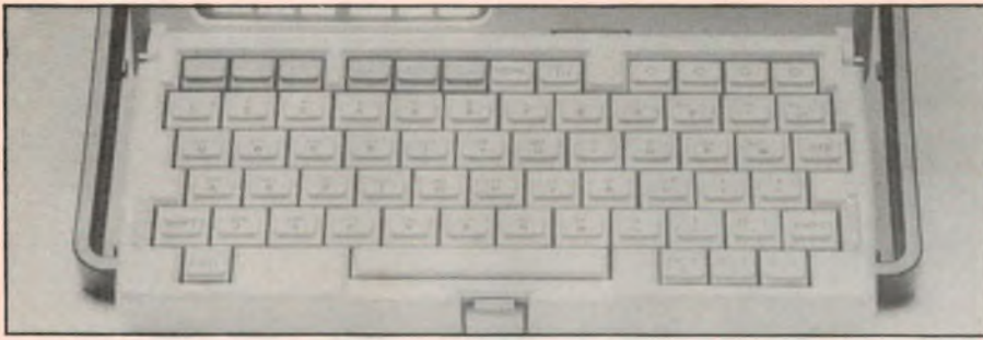
A closer look at the HP 4951C's flip-down keyboard. Unlike most computer keyboards, it can be used to generate virtually any data code.
