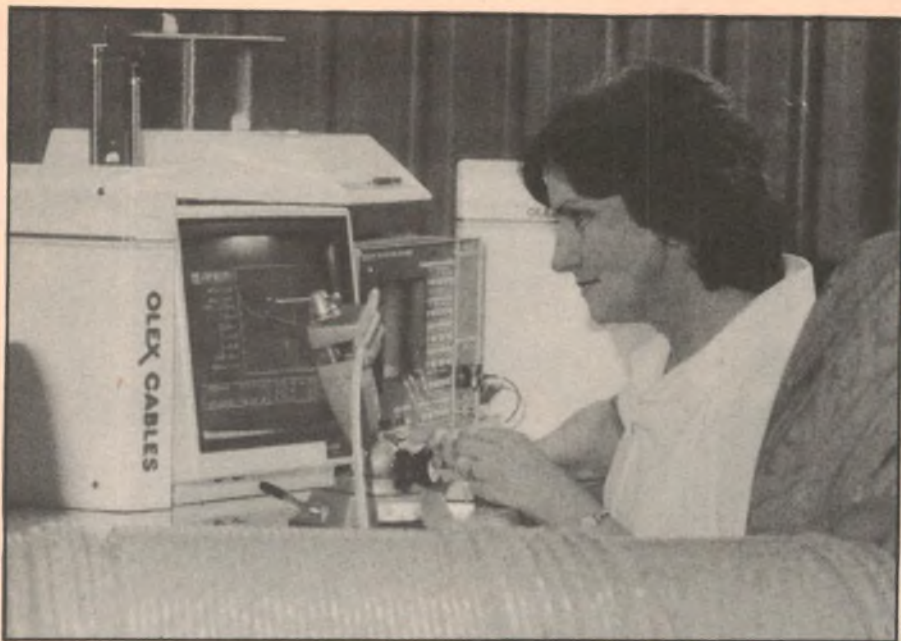
Testing an optical fibre cable for discontinuities, using an optical time-domain reflectometer or "TDR". (Courtesy Olex Fibre Optics)
