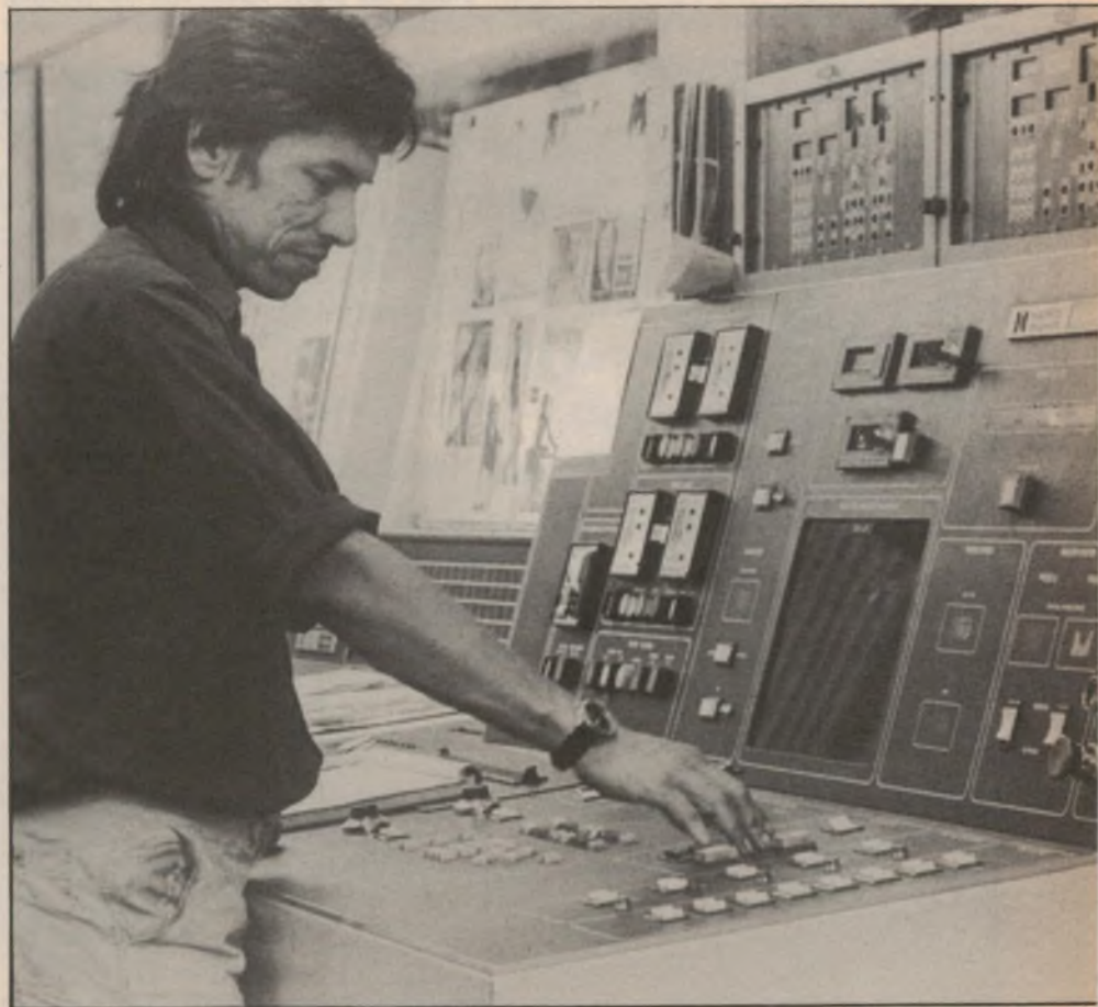
Almost all of the press' functions can be controlled from the central console area.
