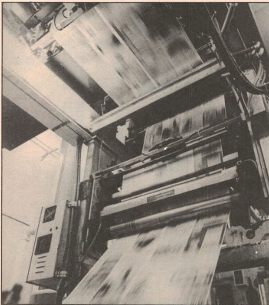
A large M-1000 press can deliver up to 44,000 complete products per hour.
