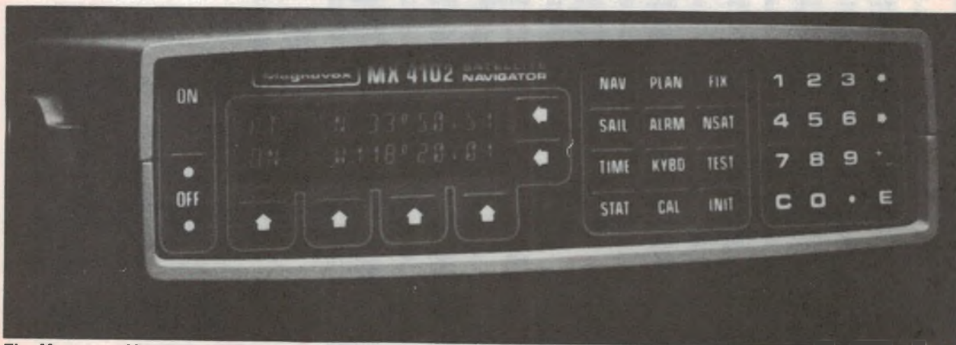
The Magnavox MX 4102 satellite navigator automatically corrects its calculation for your location each time a satellite passes overhead, and will interface to your gyrocompass and speed log. (Courtesy Coursemaster Autopilots)
