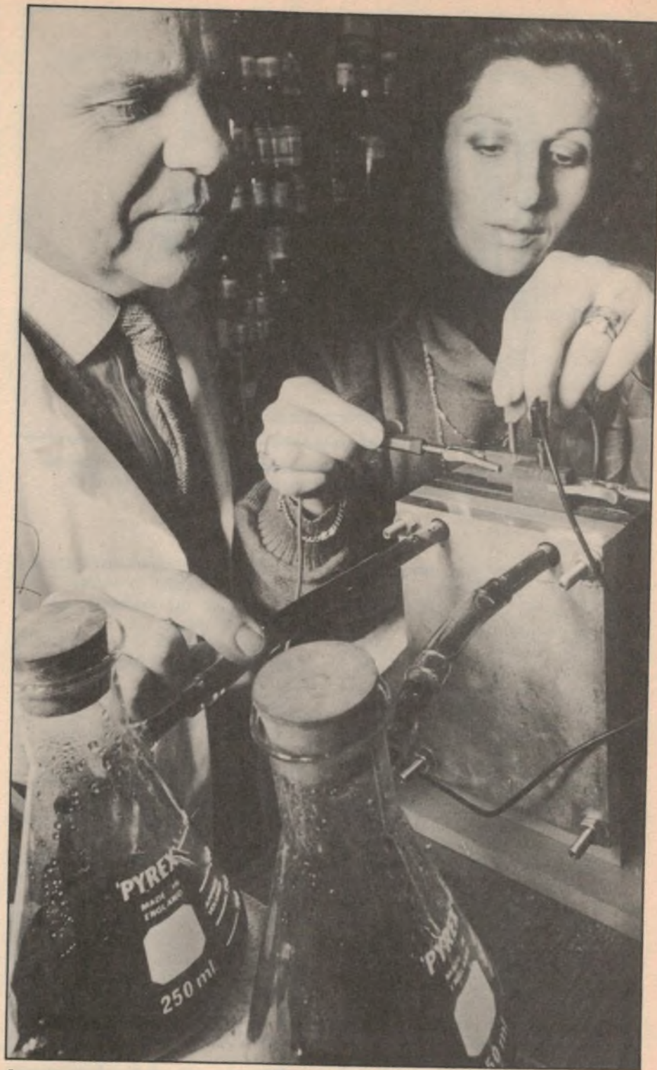
Dr Maria Skyllas-Kazacos and Dr Miron Rychcik with an experimental vanadium redox cell.
