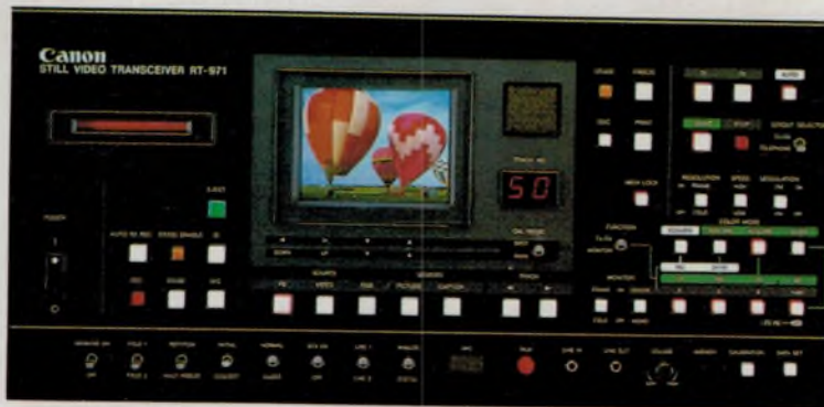
Above: The transceiver used to send the new still video pics over the telephone network. Below: Sample pics, shown actual size.
