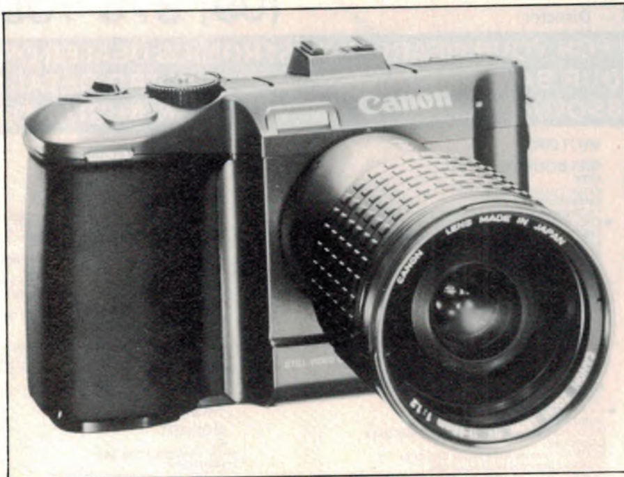
Canon's new still video camera is a little larger than a 35mm SLR, and uses 2" microfloppy magnetic disks instead of film.
