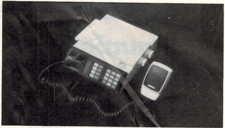
Uniden's MC-724 VHF transceiver provides 90-channel programmable scanning, 25W output. (Courtesy Dick Smith Electronics)
