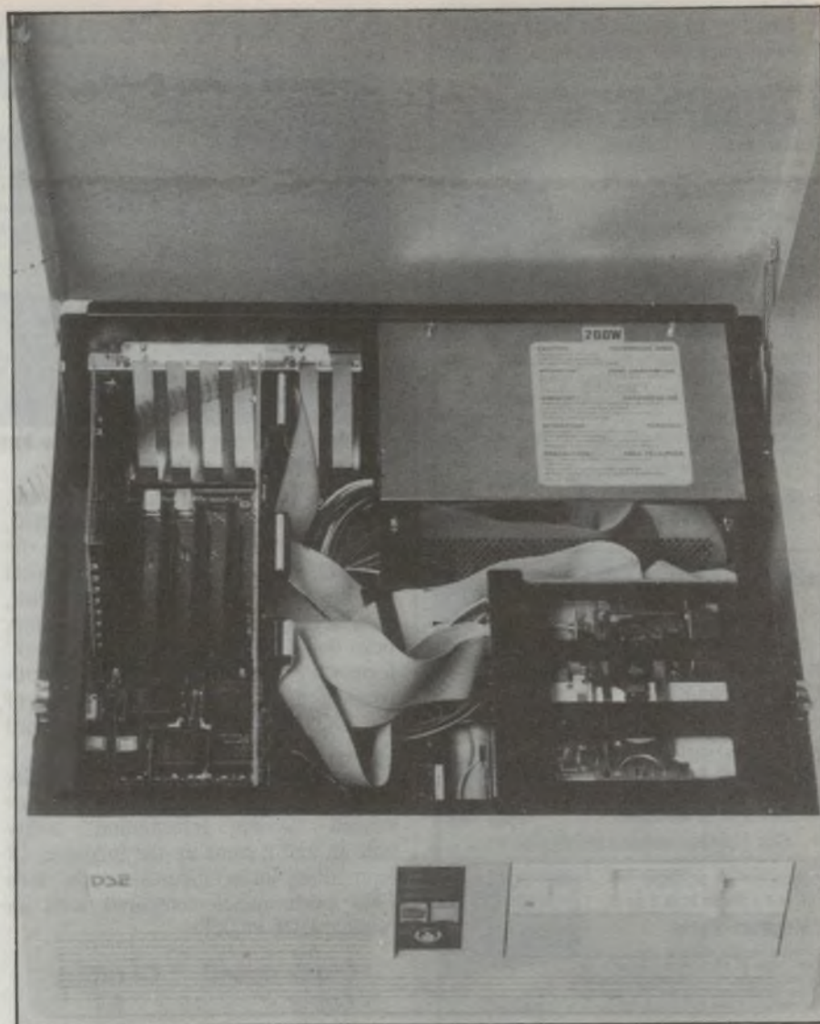
A look inside the case of the completed computer, before fitting the rear dress plates over the blank card slots.
