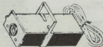
ULTRASONIC BURGLAR ALARM SYSTEM
