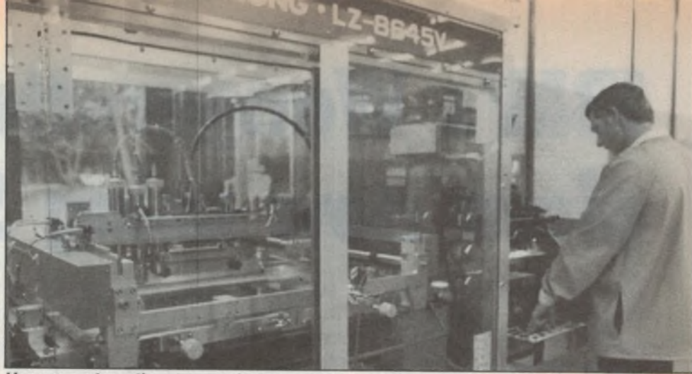
Here an automatic screen printing machine applies solder paste to the raw planar boards, before the components are placed.
