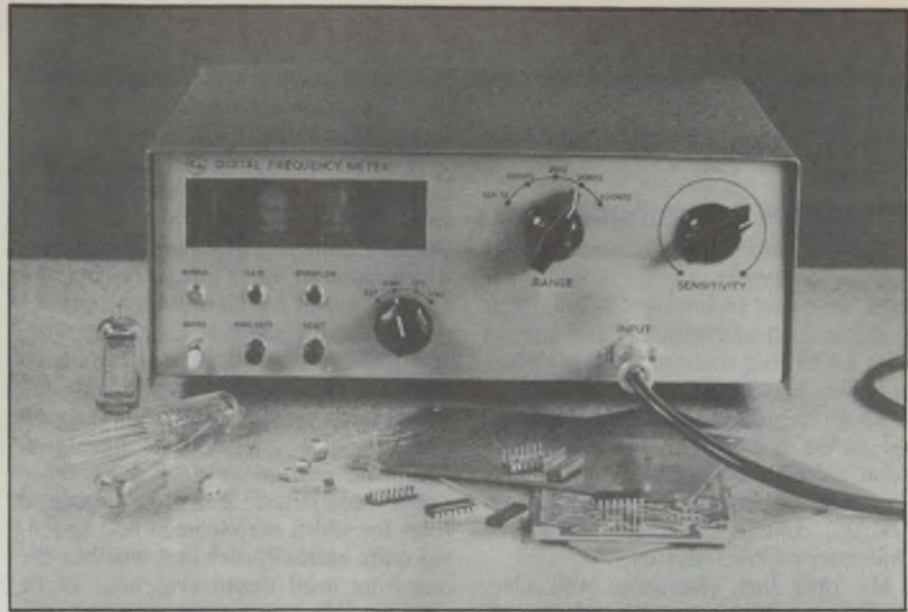
Our first digital frequency counter project, which appeared in the issues for February-June 1970. It used gas discharge tubes for readout, with a mixture of RTL, DTL and ECL ICs.
