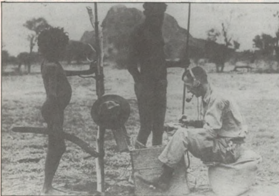
Bush padre Rev Kingsley Partridge sending a telegram to Cloncurry from outback central Australia in 1934, using Traeger's 8XP portable pedal set.
