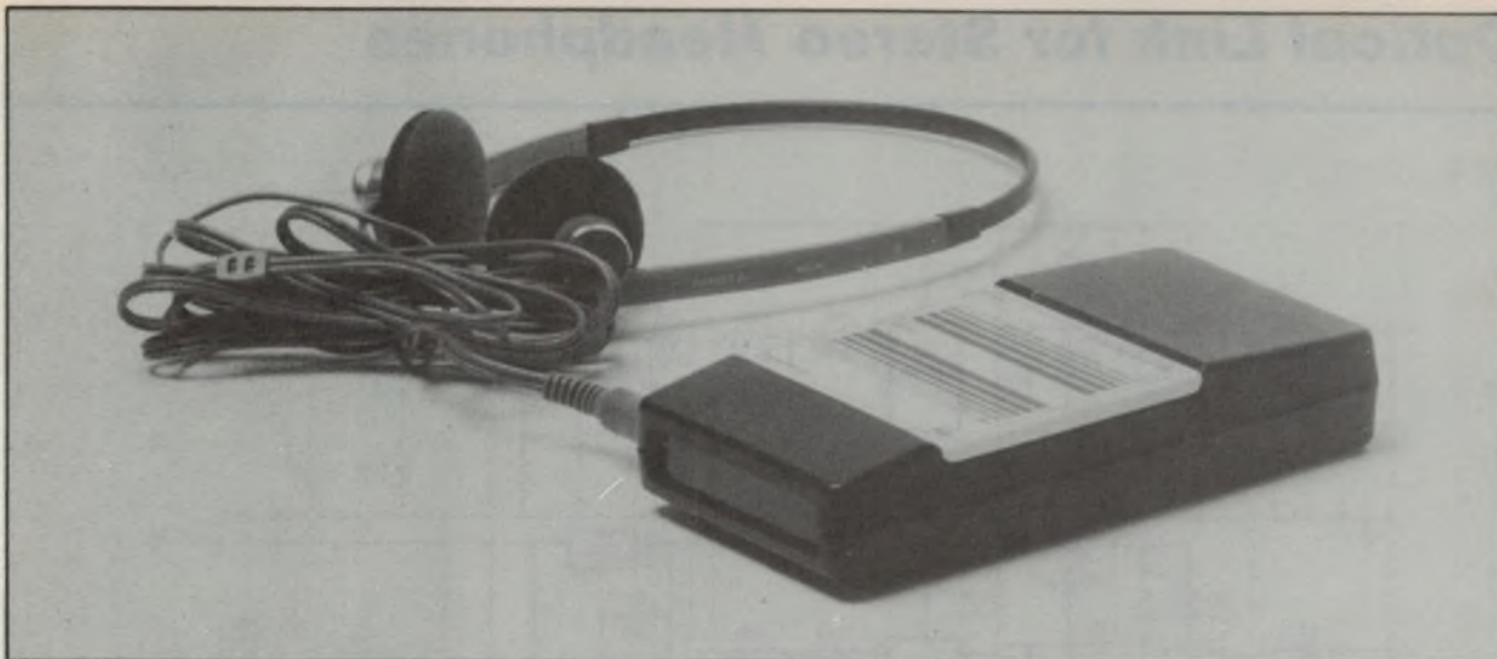
The receiver unit, with typical lightweight headphones. It runs from a standard 9V battery.
