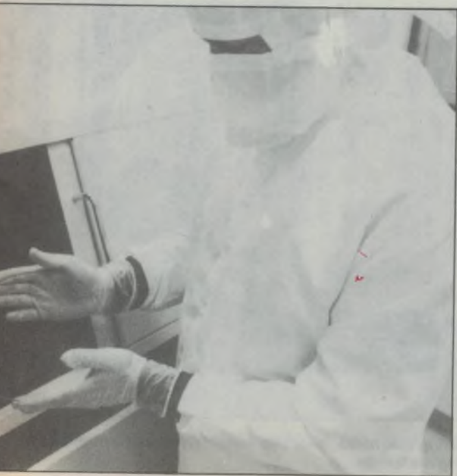
Above: Putting a polished glass master disc into the 18-stage automated cleaning machine. This uses water purified to 18 megohm resistivity.
