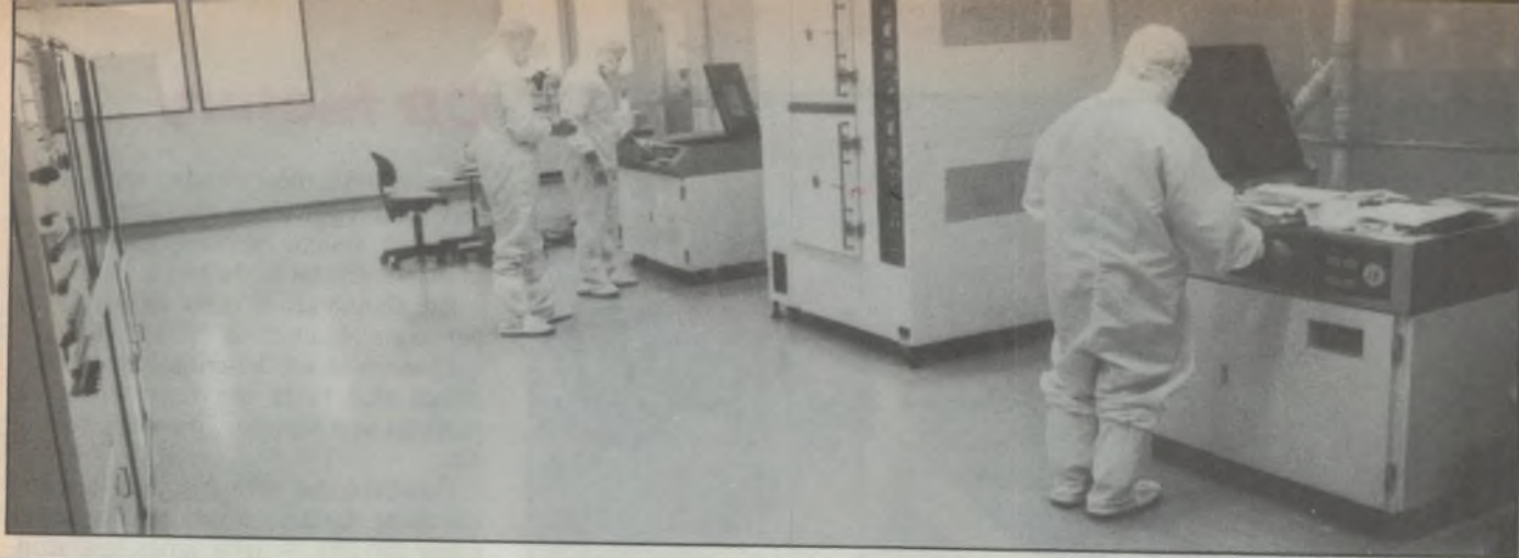
Above: A view of the master disc preparation area. The photoresist spinner/applicator is at rear, with the curing oven and developing machine to the right.
