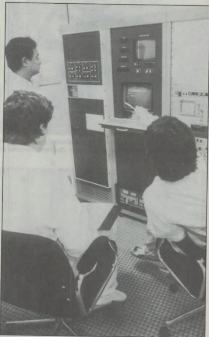
Above: Sony engineers training a Disctronics engineer on operation of the DMC-1200 laser recording electronics. The source is a PCM digital master tape.
