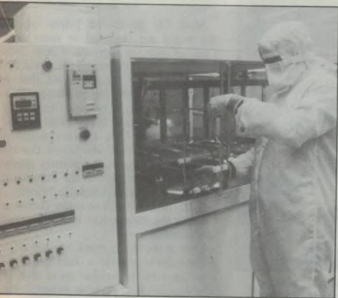
Above: Putting a polished glass master disc into the 18-stage automated cleaning machine. This uses water purified to 18 megohm resistivity.
