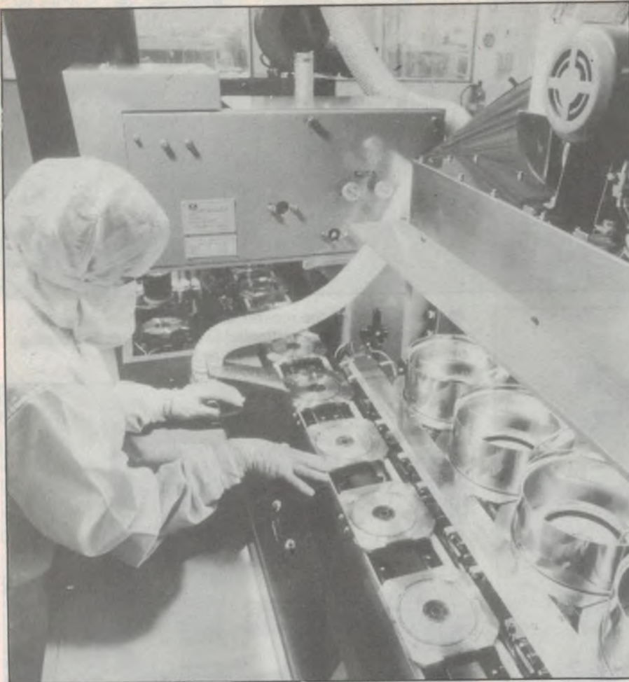
Above: Checking operation of the automated top-coating machine, which applies the clear protective acrylic over the metallisation of newly pressed compact discs.
