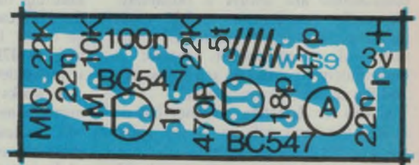
Below: The PCB overlay diagram, showing exactly where everything goes. Be careful with the orientation of the two transistors.
