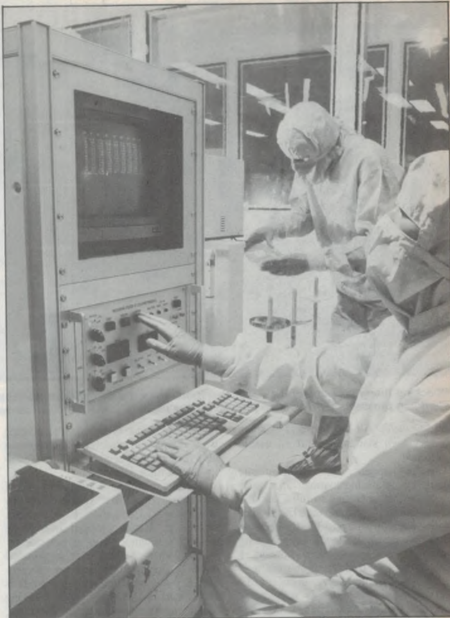
All compact discs products at Disctronics are subjected to rigorous quality control, using computer-controlled test equipment. The manufacturing yield rate is frequently as high as 95%.
