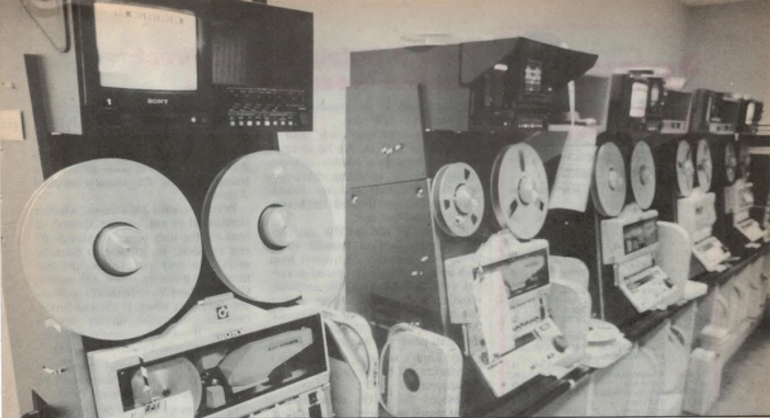
Above: Some of Sky Channel's bank of VTRs, used for program recording and editing.
