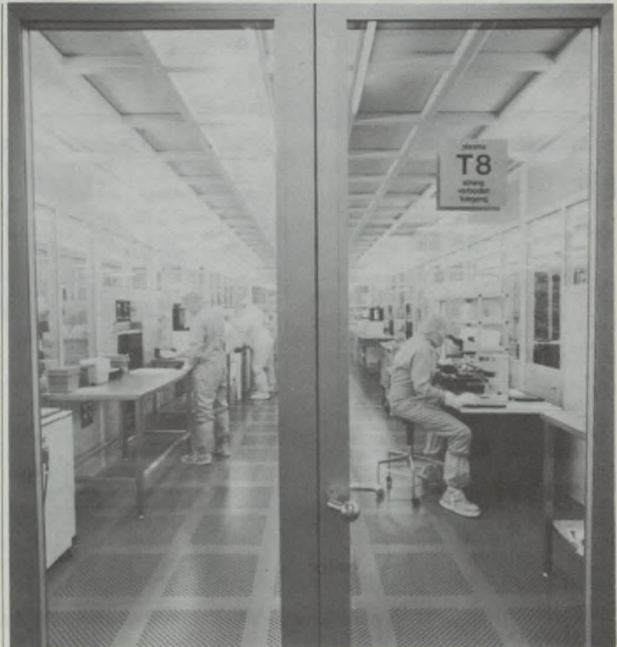
Above and below: Two views inside the Class-35 cleanroom production area of the new Submicron IC Centre. This comprises only about 7% of total building floor area.
