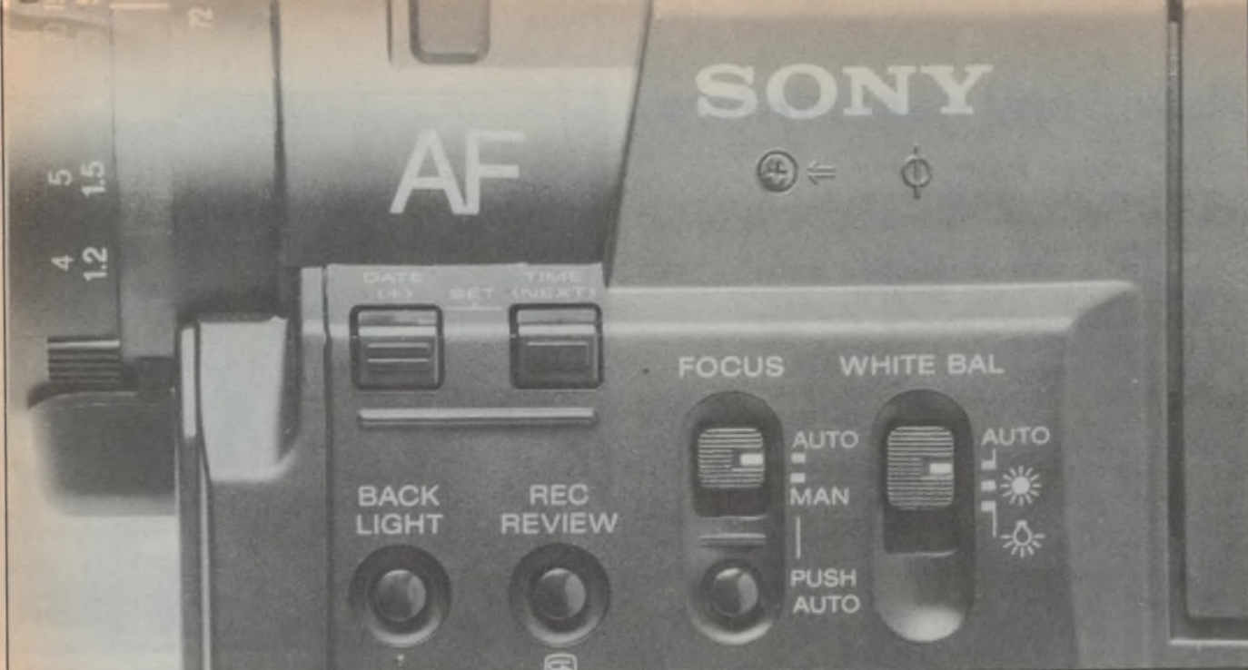
A close-up of the V50E camera control panel, showing the date and time stamping buttons.
