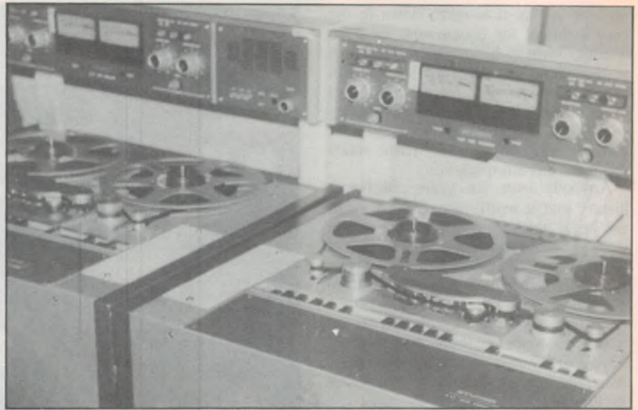
Two of the Studer recorders used by the ABC in Hobart. These machines were equipped for stereo working, ready for the change to stereo when ABC Radio moved to its new Hobart headquarters.
