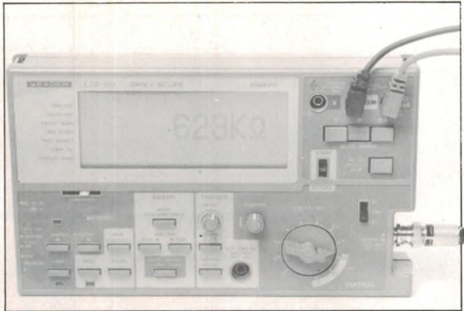
In DMM mode, the LCD-100 has large easy to read digits 15mm high. Contrast is somewhat better than this shot suggests.
