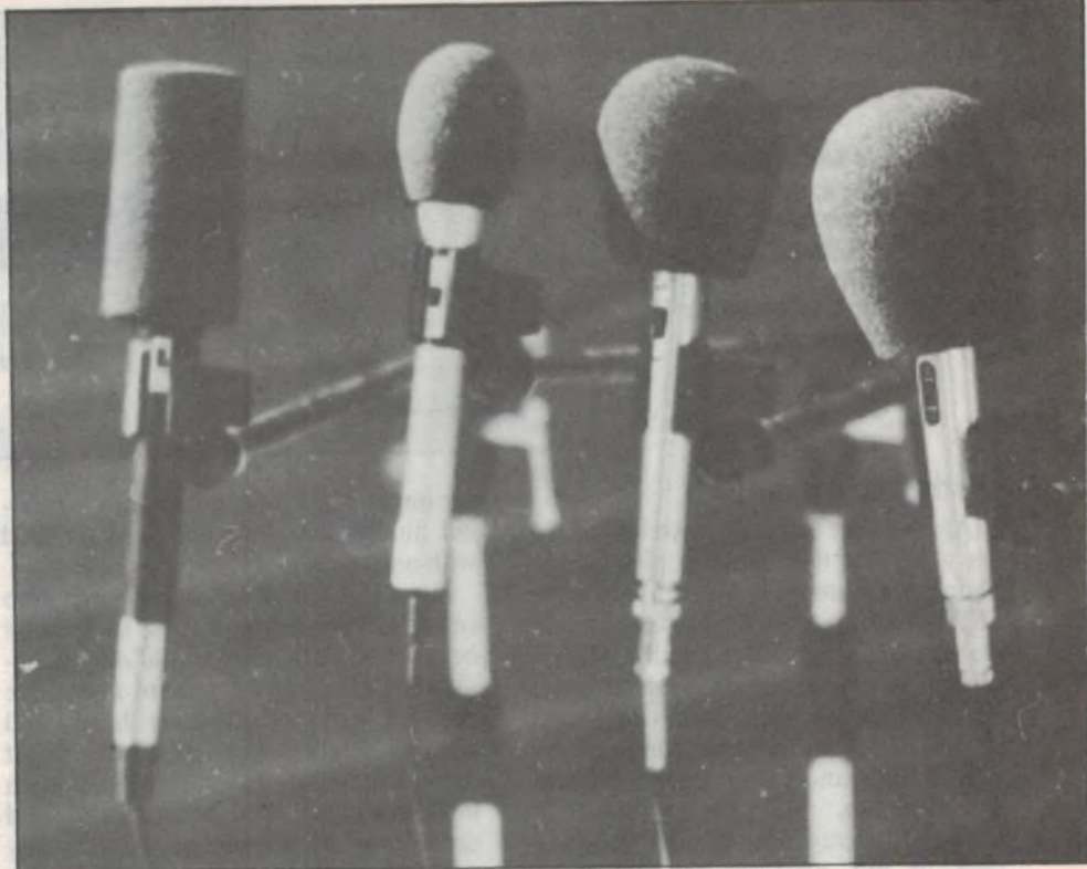
For outdoor use, microphones should have a good windshield. Foam type windshields as shown here must be snug fitting.
