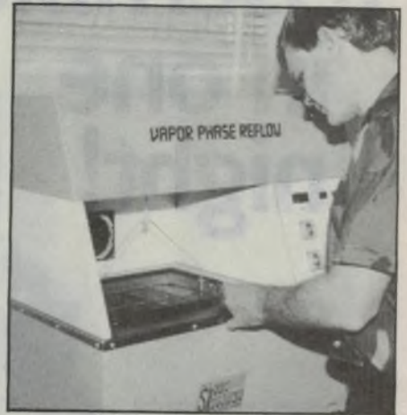
A Surf Systems VP-300 vapour phase reflow station in use at Cochlear Pty Ltd, maker of bionic ear implants.
