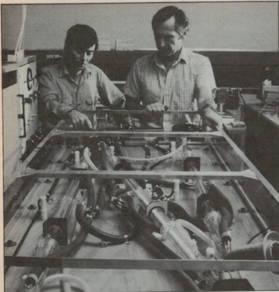
CSIRO scientists Lew Whitbourn (left) and Dick Phillips showing during testing of the laser's power supply and current control systems before the telescope optics were added. The rotating polygon mirror is just under Dick Phillips' hand, with the output end of the laser just out of picture at bottom left.
