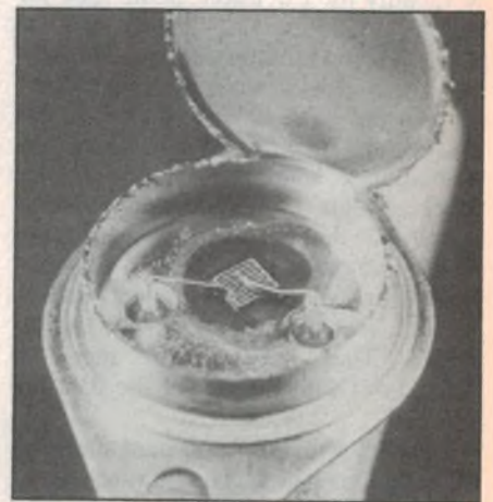
Inside two typical bipolar transistor packages, showing the actual chips and the small bonding wires used to connect to them. The TO-18 device at left is about 10 times actual size.
