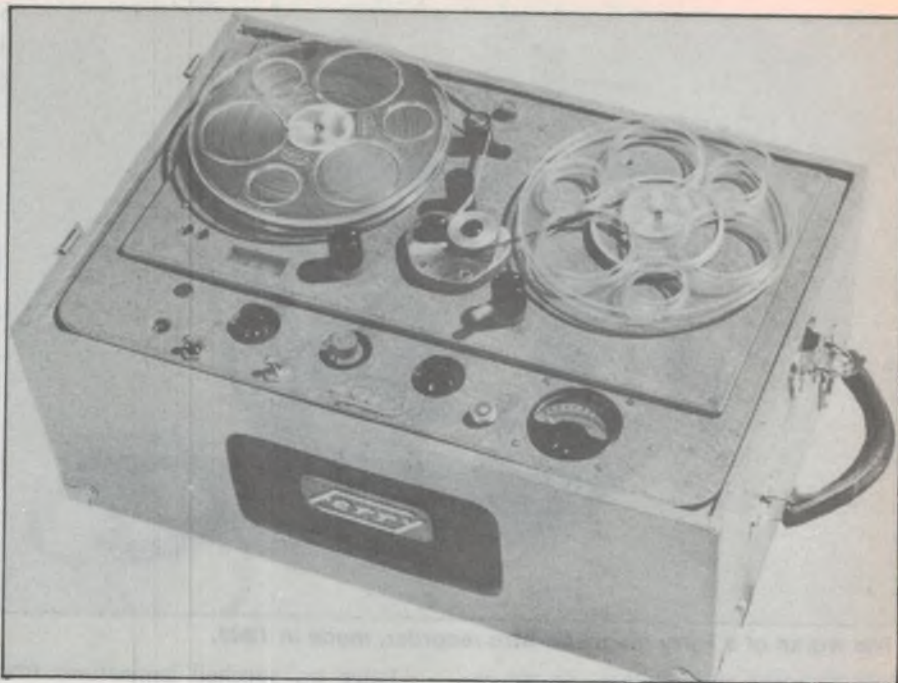
One of the first 12 Ferry magnetic tape recorders, made in 1950. These first machines were full track and ran at 7.5ips. They used DC recording bias, and had no "fast forward" facility.
