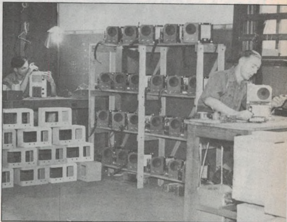
Making 5-valve mantel radios in 1947. Jack Ferry himself is at right, doing the alignment. About 400 were exported to Japan!
