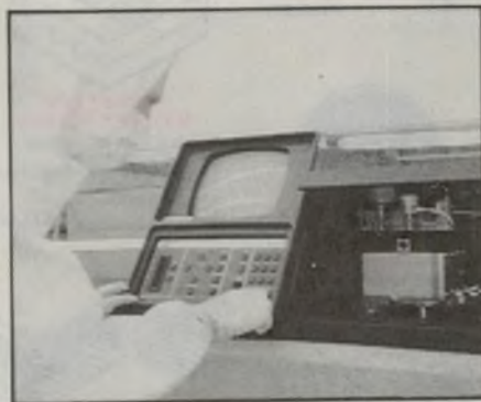
One of the three LAM Research plasma etchers used in wafer fabrication. One is used for etching metal, the other two for oxide and polysilicon respectively.
