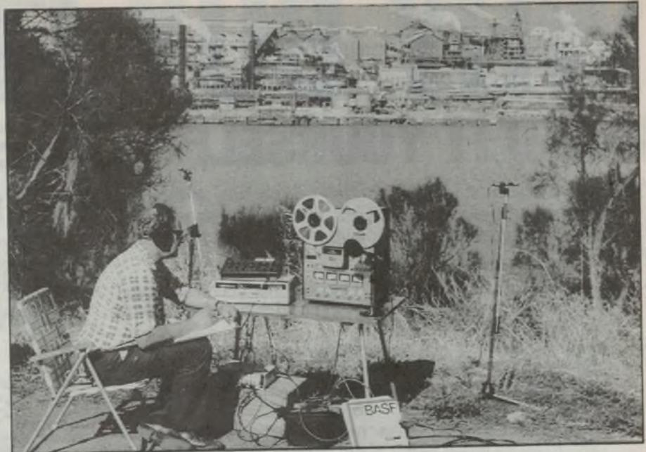
The author recording stereo sound effects on location. The two recorders are powered from a pair of 12V batteries via a 300VA inverter.
