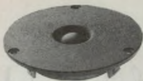
Fig.1: The tweeter used is the Vifa D19TD-05-08, a 19mm dome type with ferrofluid for cooling and damping.
