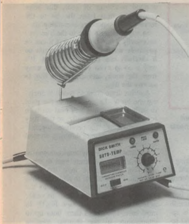
Above left is Dick Smith Electronics' reasonably priced soldering station, with meter readout of temperature. Above right is the Royel double-iron station, with its twin soldering irons.
