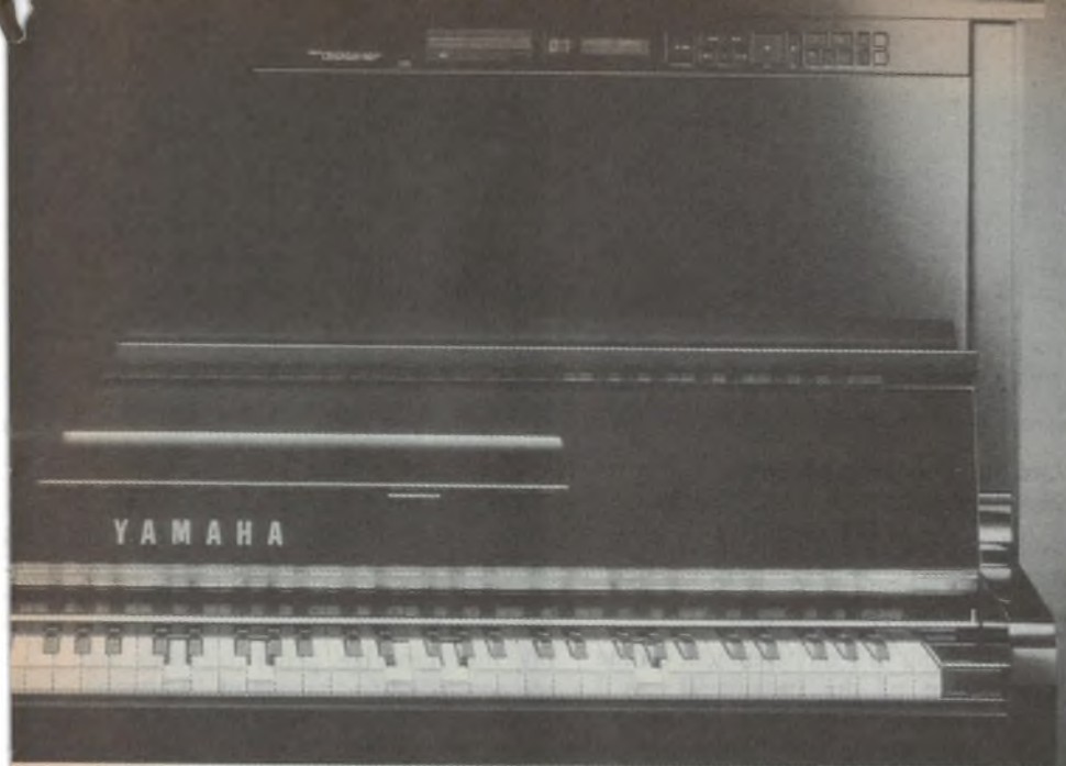
The Disklavier's disk drive, display panel and controls are discretely housed at the top of the piano case.
