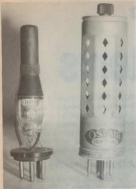
Fig.2 (above): On the left is the MH4 Catkin triode with base and cover removed. Note the resemblance to the CAT9. The VMS4 variable-mu RF amplifier is at right.
