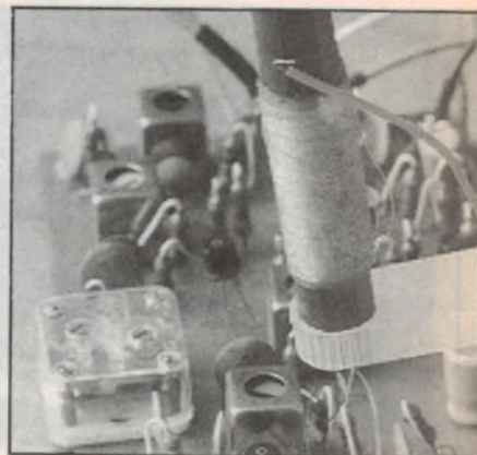
Fig.1: The first tuned circuit of this radio consists of the ferrite cored coil in the centre and the miniature tuning capacitor at lower left.
