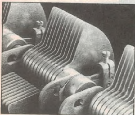
Fig.5: Close-up of a fairly large three gang tuning capacitor for tuning the broadcast band. All three variable 50 – 350pF sections are on a common shaft.
