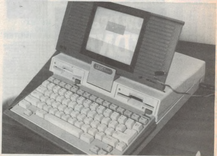
Active matrix in colour. Unfortunately our black and white reproduction doesn't show the effect, but this display is actually showing five colours.
