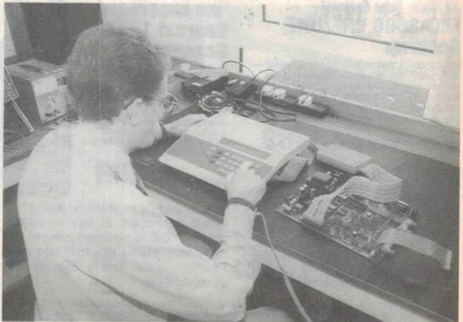
Fault finding using high tech! Here the Polar B3T micro tester is being used in a microprocessor-based circuit.
