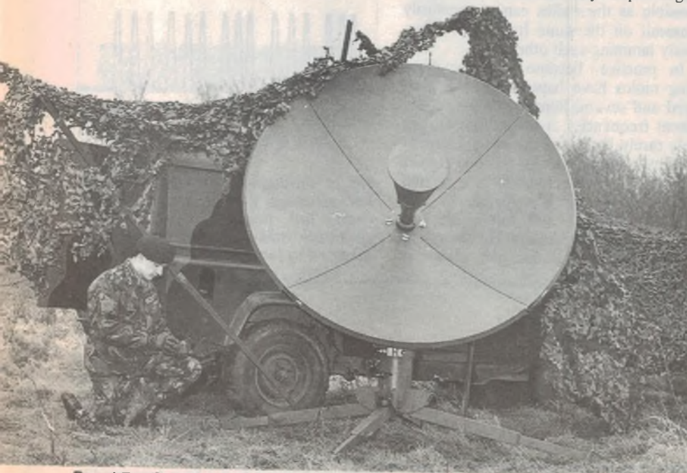
Racal-Tacticom's new TSC 501 satellite comms terminal. Two men can have it set up and running in less than 10 minutes.
