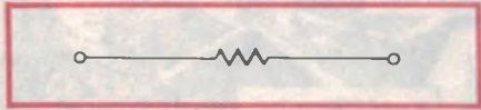
Fig.1: Most of us think of a copper wire as simply a low-value resistor...
