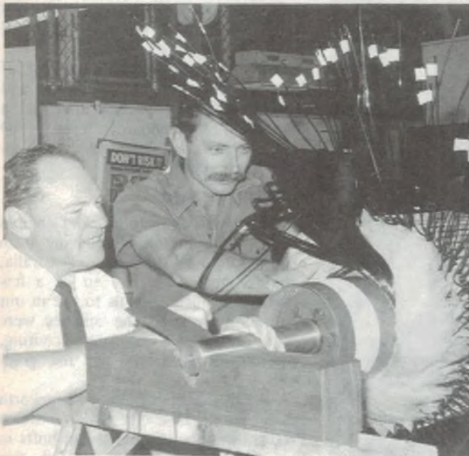
Ron Greer, who designed the recreated dynamos for the museum, looks on as one of the armatures is wound and assembled by mechanic Dick Cooksey in the PCCC workshops.
