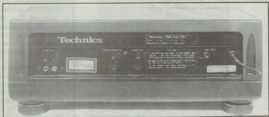
Rear view of the player, showing the wired remote input and subcode output connectors.
