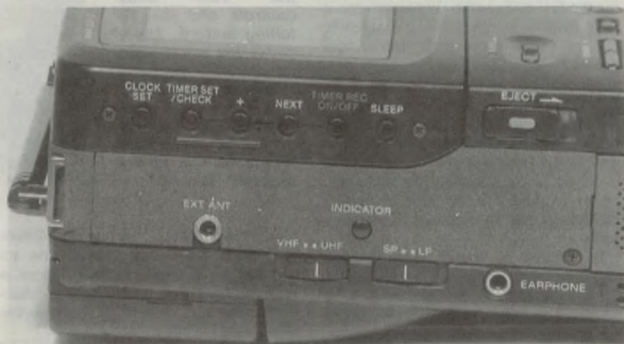
Above: A look at the controls and connectors along the left-hand side of the GV-8. The LCD screen tilts up for viewing.
