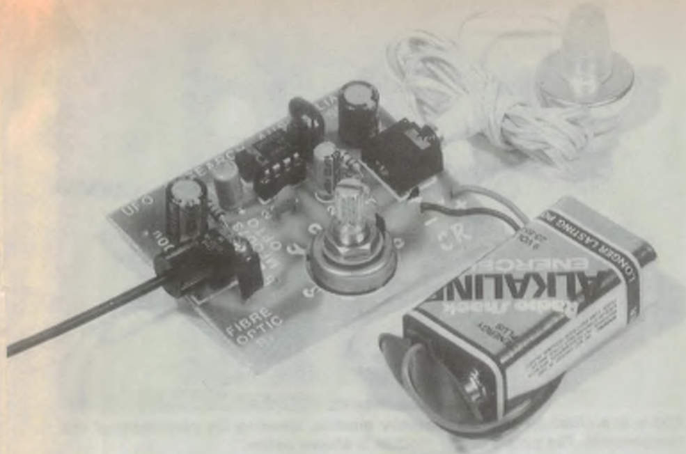
The receiver module, which can be used to drive either headphones or a small speaker. The opto detector is at lower left.
