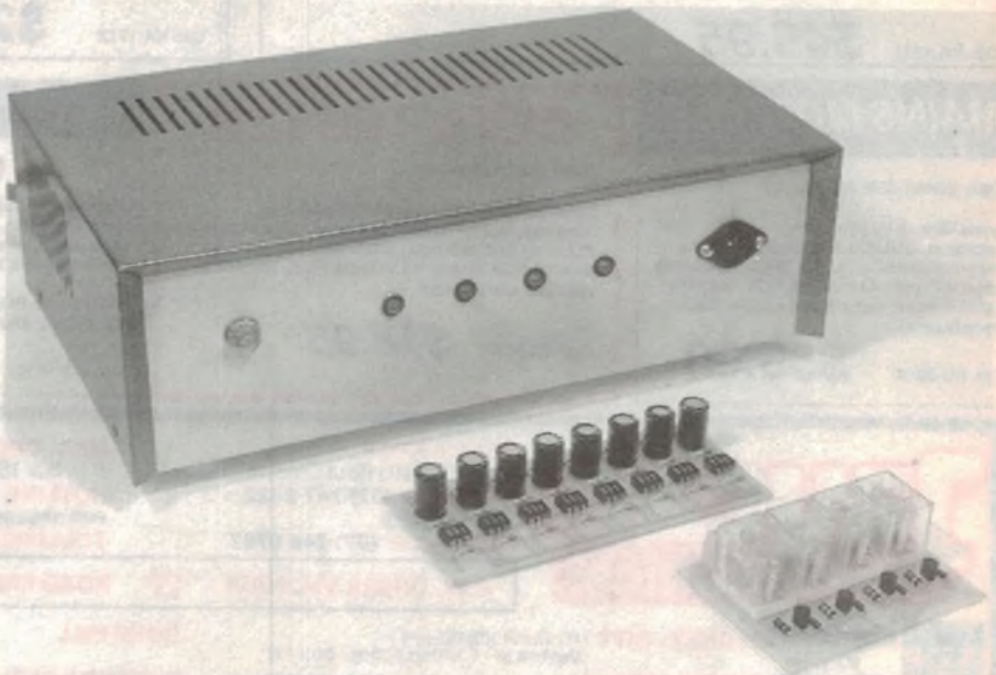
The three completed boards. At the rear is the triac board in its enclosure, with the relay board in front and the input board in the middle.
