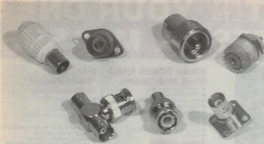
RF connectors. Top left shows the types used for TV antenna connections, top right the PL-259 plug and the SO-239 socket. Underneath are examples of the BNC range of connectors.
