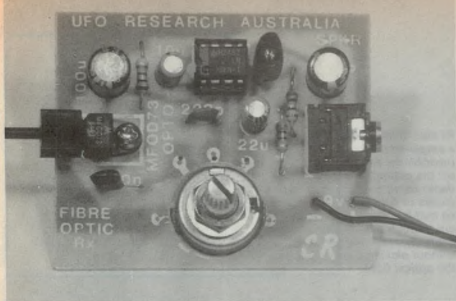
And here is the receiver module (above), again showing the component placement. Be careful with the polarised parts!
