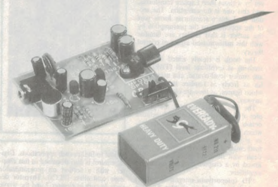
The transmitter module, which includes an on-board electret microphone – but also a socket which allows you to use an external mic instead.
