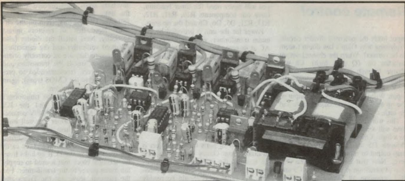
The mains interface can drive up to four 240V appliances, and can also serve as the power supply for the rest of the remote control system.
