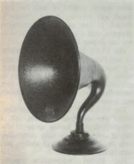
An American Atwater Kent model L. It has a spacing adjustment collar under the base.
