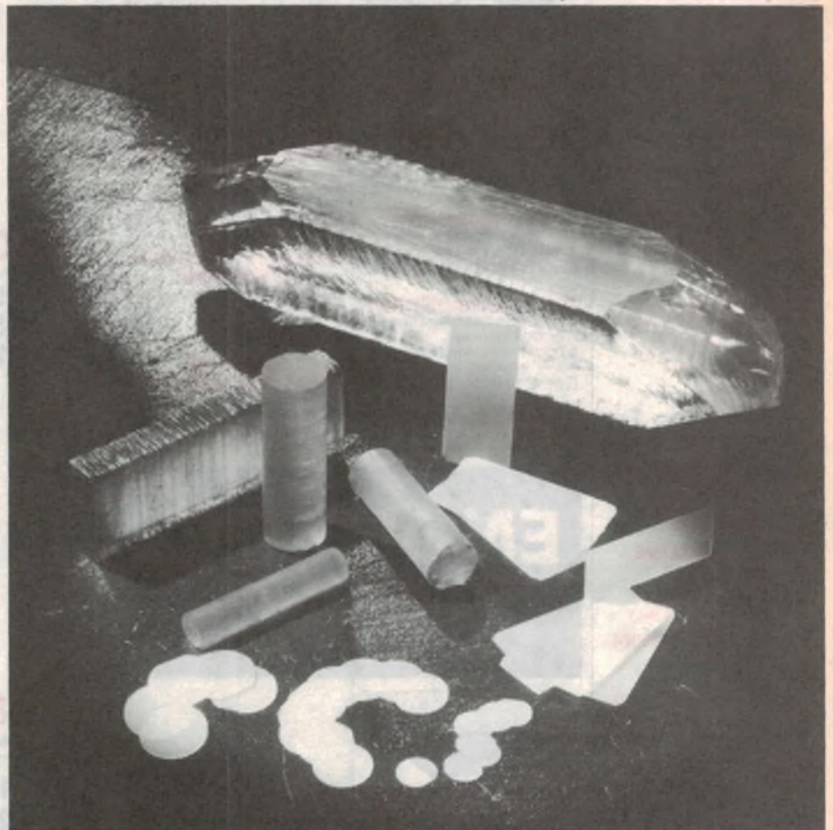
Various stages in the manufacture of a quartz crystal, from a large raw crystal in the background to sawn disks in the foreground. (Courtesy Hy-Q International)
