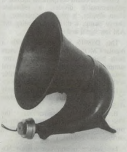
A German 'N&K' horn; the adjuster is at the end of the driver unit.
